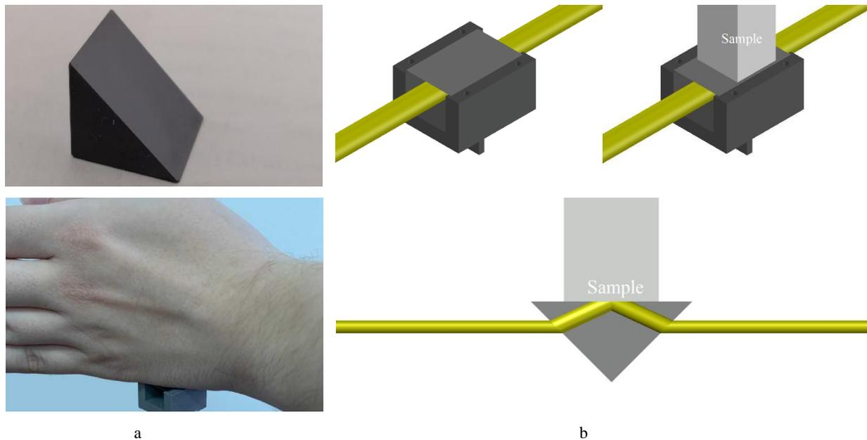
Figure 2 - Prism ATR (a), the reflection scheme (b)
