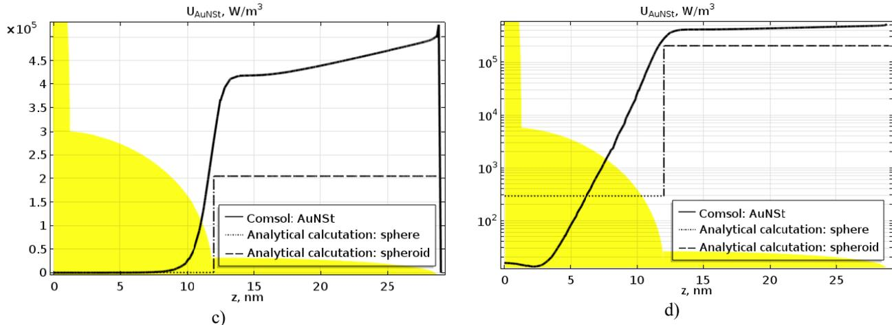
Figure 2. Distribution of the bulk density of the absorbed power ( $U_{\text{AuNSt}}$ ) for the nanostar model in Fig. 1(a): a and b – along the  $x$ -axis and the  $y$ -axis; c and d – long the  $z$ -axis (along the polarization vector of the incident field) in linear and logarithmic scale, respectively. The points and the dotted line represent the distribution of  $U_{\text{AuNSt}}$  according to an approximate analytical estimate.
