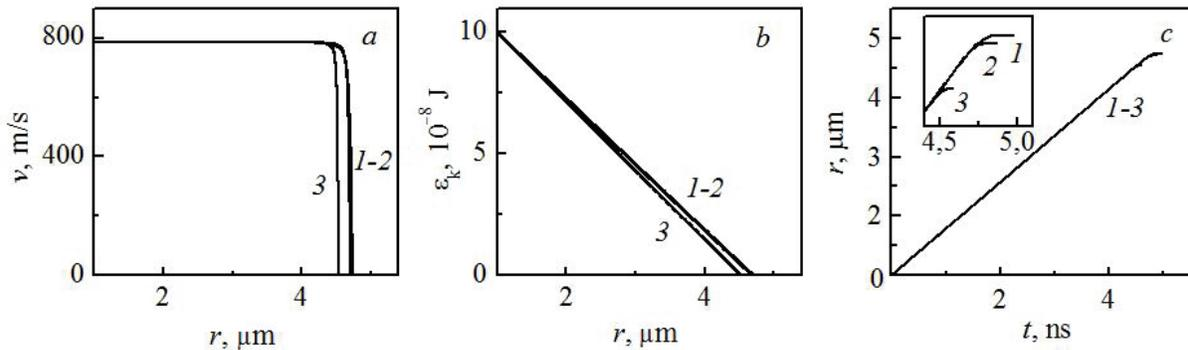
**FIGURE 2.** The dependence of the dislocation velocity  $v$  (a), the kinetic energy per unit length of the dislocation  $\epsilon_k$  (b) on the dislocation path length, and the dependence of the dislocation path length  $r$  on the time of its path (c) under different dislocation densities  $\rho$  in lead,  $\text{m}^{-2}$ : 1 –  $10^8$ , 2 –  $10^{11}$ , 3 –  $10^{13}$
