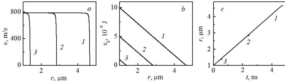
**FIGURE 3.** The dependence of the dislocation velocity  $v$  (a), the kinetic energy per unit length of the dislocation  $\varepsilon_k$  (b) on the dislocation path length, and the dependence of the dislocation path length  $r$  on its path time at different values of the initial kinetic energy  $\varepsilon_k^{(0)}$ ,  $J$ : 1 –  $10^{-7}$ , 2 –  $5 \cdot 10^{-8}$ , 3 –  $10^{-8}$
