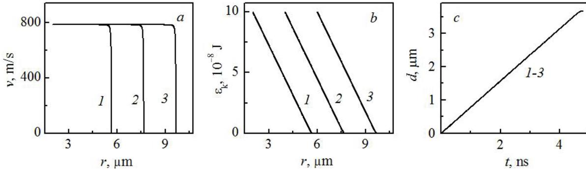
**FIGURE 1.** The dependence of the dislocation velocity  $v$  (a), the kinetic energy per unit length of the dislocation  $\epsilon_k$  (b) on the dislocation path length, and the dependence of the dislocation path length  $r$  on its path time (c) with a different diameter of the contact spot, micron: 1 – 2, 2 – 4, 3 – 6
