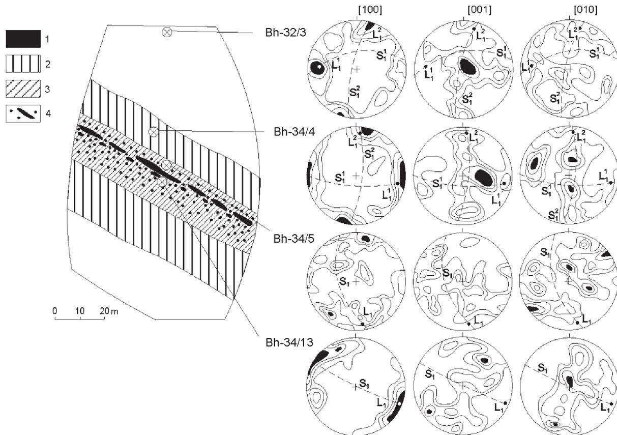
Figure 2. Optic orientation of olivine in chromite-bearing ultramafic rocks from the Barkhatny Massif: 1-3 – types of deformation microstructures: 1 – protogranular; 2 – protogranular – protogranular - parquet-like; 3 – leystic, mosaic, mosaic-leystic; 4 – zone of chromite mineralization.
