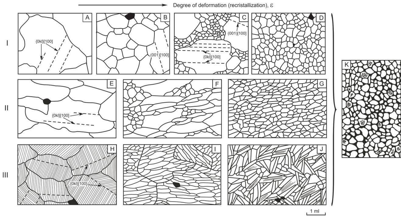
Figure 1. Deformation types of olivine microfabrics according to (Krasnova, 2005): A – protogranular; B – mesogranular; C – porphyroclastic; D – mosaic; E – leystic; F – porphyroleystic; G – mosaic-leystic; H – protogranular-cleavaged; I – parquet-like; J – pseudospinifex; K – regenerated.
