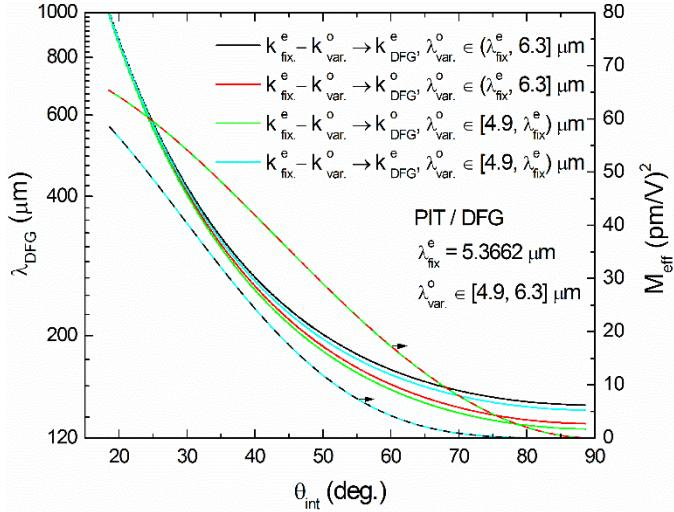
Fig. 3. Phase matching curves for I and II type down-conversion of nonselective CO laser lines in PIT: 5.3662 μm is the most powerful emission line; longer (up to 6.3 μm) and shorter (down to 4.9 μm) wavelengths pump was considered. Presented data, not possibility, are limited by 1000 μm.
