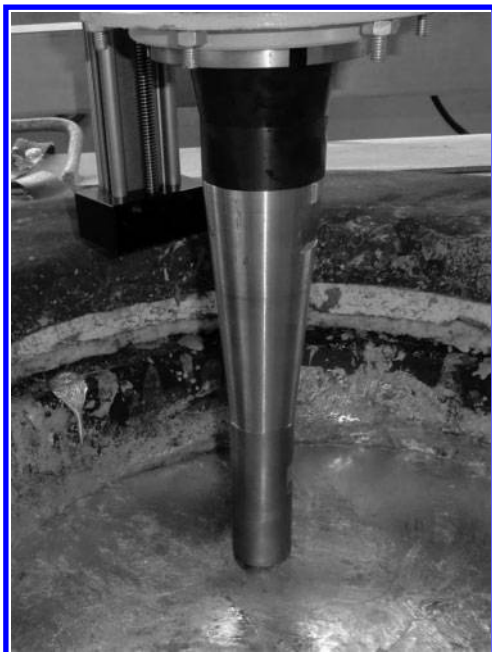
7 Photograph of ultrasonic transducer and sonotrode inside 150 kg crucible during degassing trials
