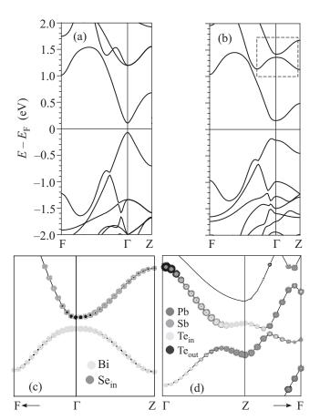
Fig. 4. (Color online) Bulk band structure of  $Bi_2Se_3$  without (a) and with (b) SOI included. (c) – Magnified view of blue dashed frame marked in the Fig. 4b with composition of the second and third conduction bands in the vicinity of  $\Gamma$ . (d) – The same for PbSb<sub>2</sub>Te<sub>4</sub> in the vicinity of Z
