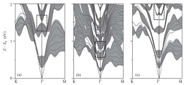
Fig. 1. (Color online) Surface electronic structure of Bi<sub>2</sub>Se<sub>3</sub> (a), PbSb<sub>2</sub>Te<sub>4</sub> (b), and Pb<sub>2</sub>Bi<sub>2</sub>Te<sub>2</sub>S<sub>3</sub> (c) above  $E_F$  as calculated by VASP. Size of red circles correspond to the weight of the states in the outermost block. The projected bulk bands is shown in green. Dashed frames mark region of the unoccupied Dirac-like surface state
