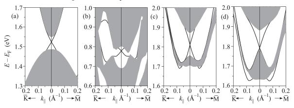
Fig. 2. (Color online) A magnified view of dashed frames marked in the Fig. 1 with CB cone in the center: (a) – Bi<sub>2</sub>Se<sub>3</sub>; (b) – PbSb<sub>2</sub>Te<sub>4</sub>; Pb<sub>2</sub>Bi<sub>2</sub>Te<sub>2</sub>S<sub>3</sub> as calculated by VASP (c) and FLEUR (d) Codes
