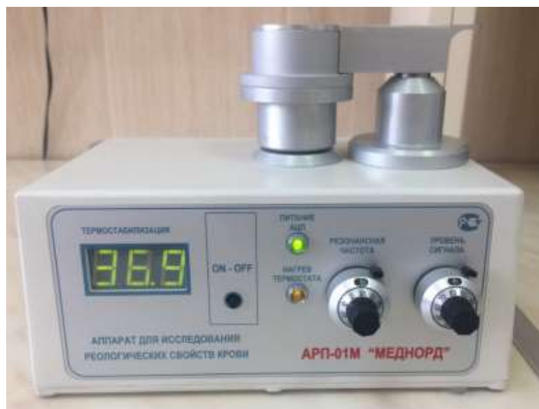
Figure 2 – Apparatus for studying the rheological properties of blood ARP-01M Mednord
