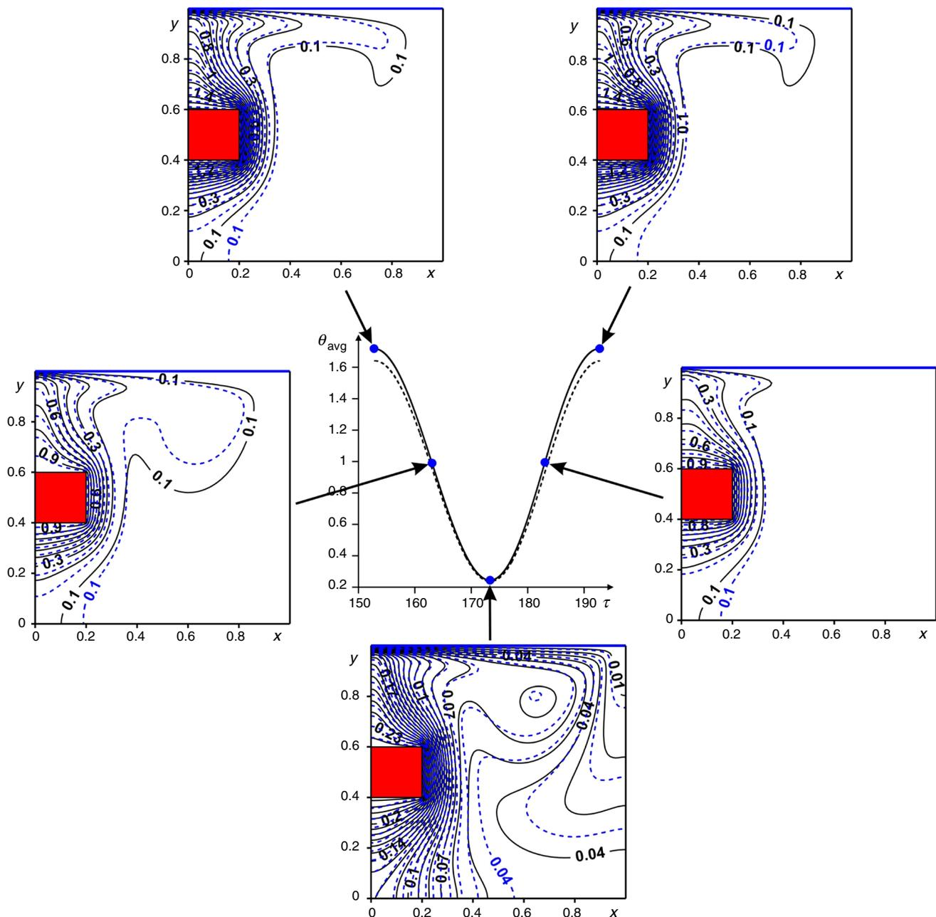
**Fig. 4** Evolution of isotherms for  $Ra = 10^5$ ,  $Re = 100$ ,  $R_d = 1$ ,  $\delta = 0.4$ ,  $f = 0.05\pi$  at  $\phi = 0.0$  (solid lines) and  $\phi = 0.04$  (dashed lines)
