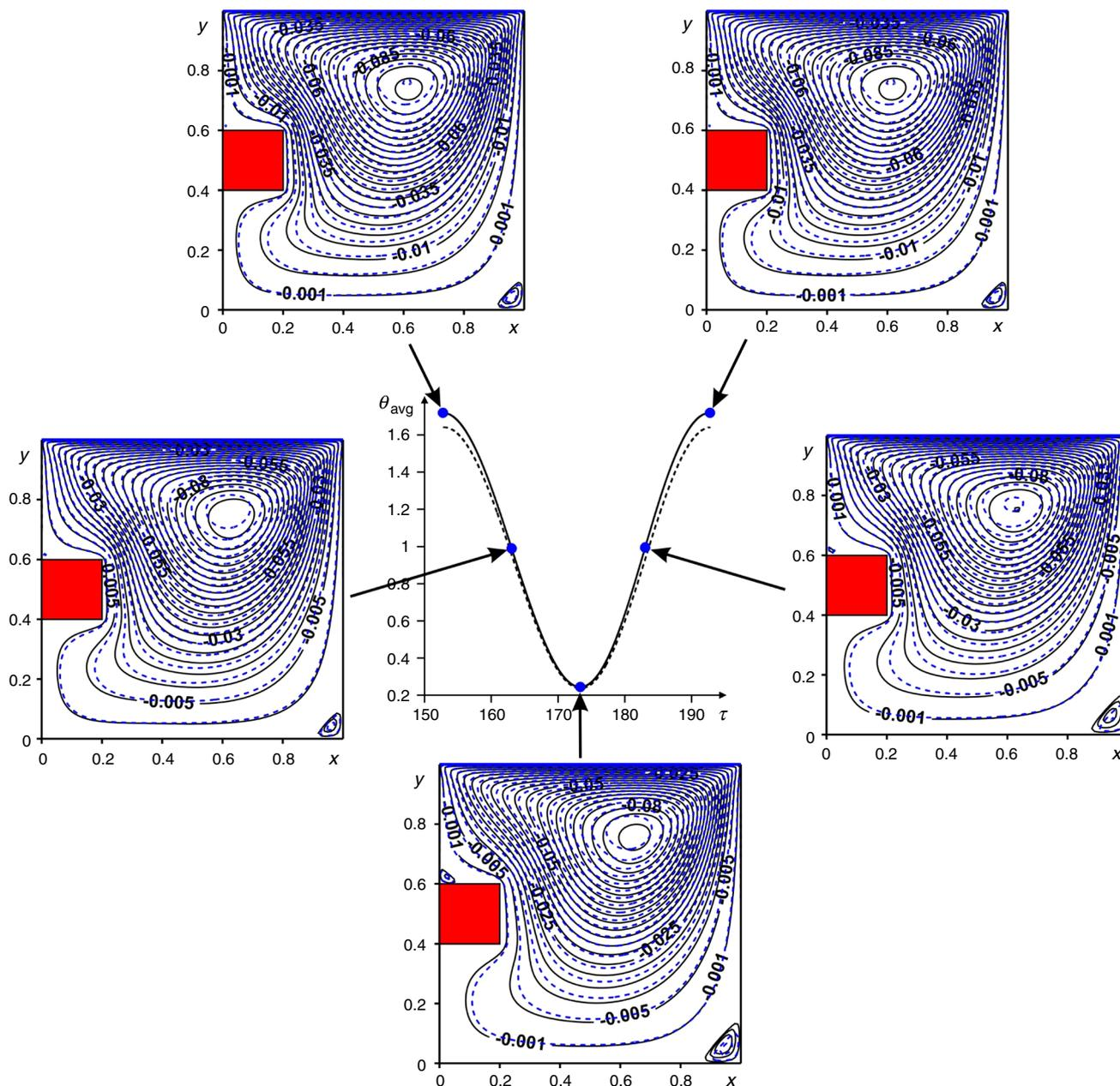
Fig. 3 Evolution of streamlines for  $Ra = 10^5$ ,  $Re = 100$ ,  $R_d = 1$ ,  $\delta = 0.4$ ,  $f = 0.05\pi$  at  $\phi = 0.0$  (solid lines) and  $\phi = 0.04$  (dashed lines)
