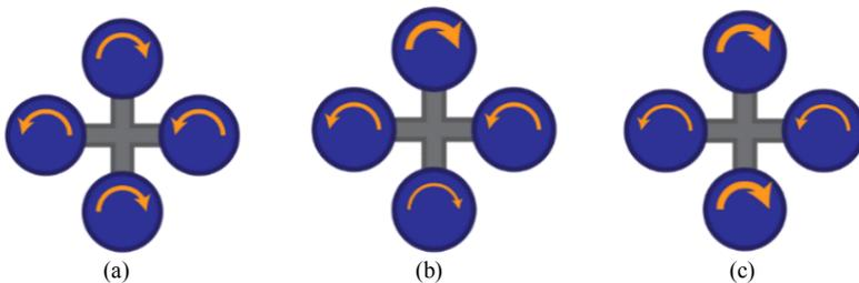
Fig. 1. Performing different movements of a quadcopter: (a) hover: all the motors have the same speed, (b) pitch or roll: one motor has higher speed than the others, (c) yaw: two motors of the same direction have higher speed than the other two motors [20]
