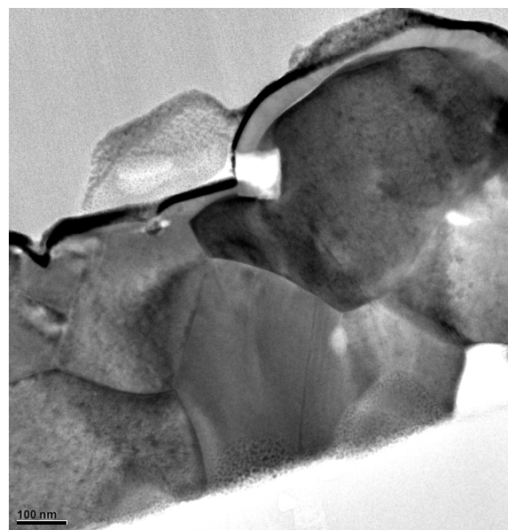
Figure 2: The microphotograph of the cross-section of the chemically deposited PbSe-based photoresistor obtained with the help of the high-resolution transmission electron microscopy
