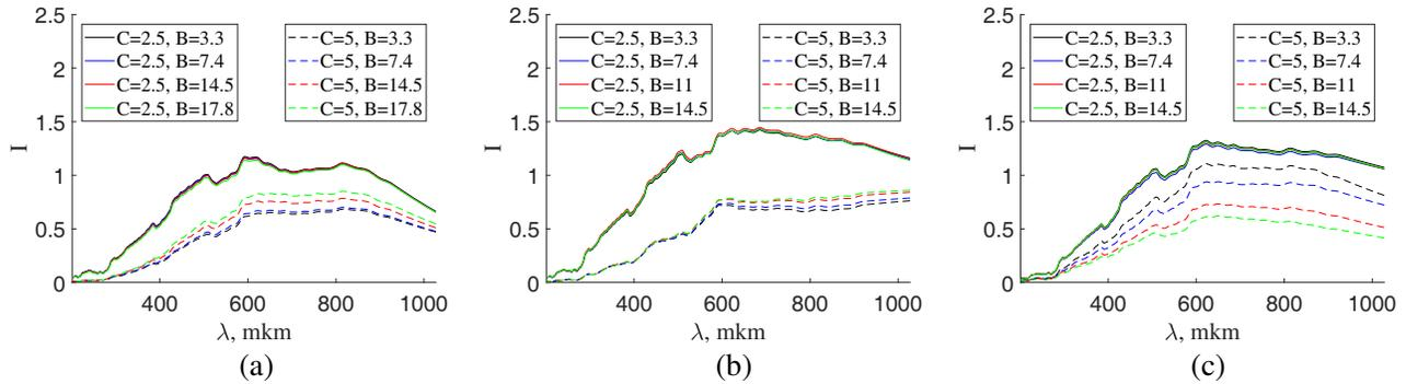
**Figure 7.** Spectra of THz signal intensity passing through MF<sub>alloy</sub> when the Helmholtz rings are located: (a) No. 1, (b) No. 2, (c) No. 3. Here  $C$  is the concentration (%),  $B$  — magnetic field induction (mT).
