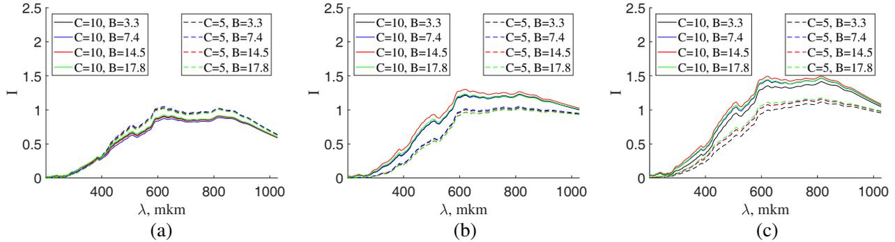
**Figure 6.** Spectra of THz signal intensity passing through MF<sub>300</sub> when the Helmholtz rings are located: (a) No. 1, (b) No. 2, (c) No. 3. Here  $C$  is the concentration (%),  $B$  — magnetic field induction (mT).
