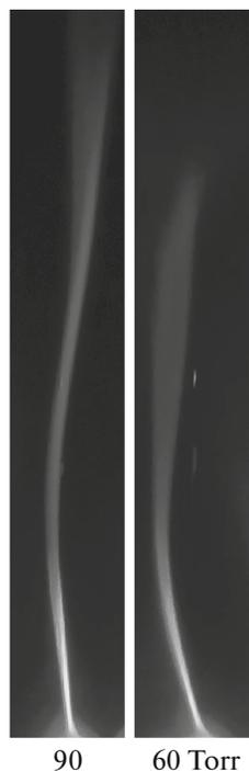
**Fig. 2.** Apokamp in air at different pressures; frame height is 25.5 cm.
