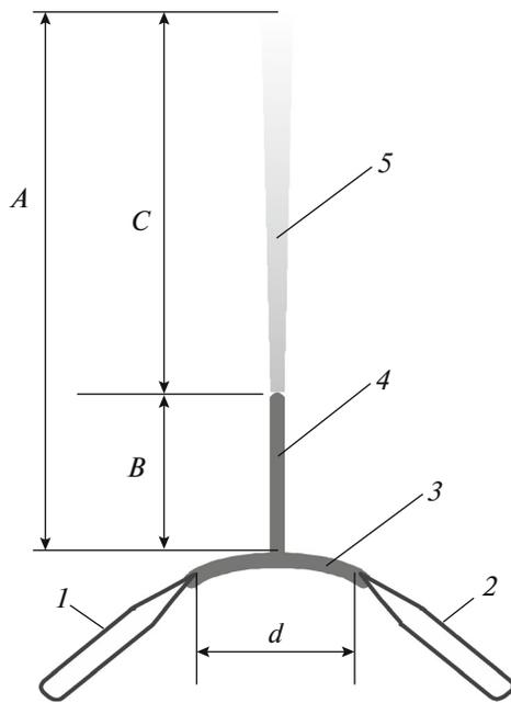
**Fig. 1.** Scheme of formation and geometric parameters of an apokamp discharge: high-voltage electrode (1); electrode at a floating potential (2); pulsed discharge current channel (3); bright branch of  $B$  in height (4); region of plasma bullets of  $C$  in height (5); discharge gap ( $d$ ); apokamp height ( $A$ ).
