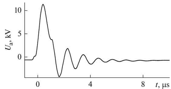
**Fig. 3.** Time variation in the voltage at the high-voltage electrode at an air pressure of 60 Torr.
