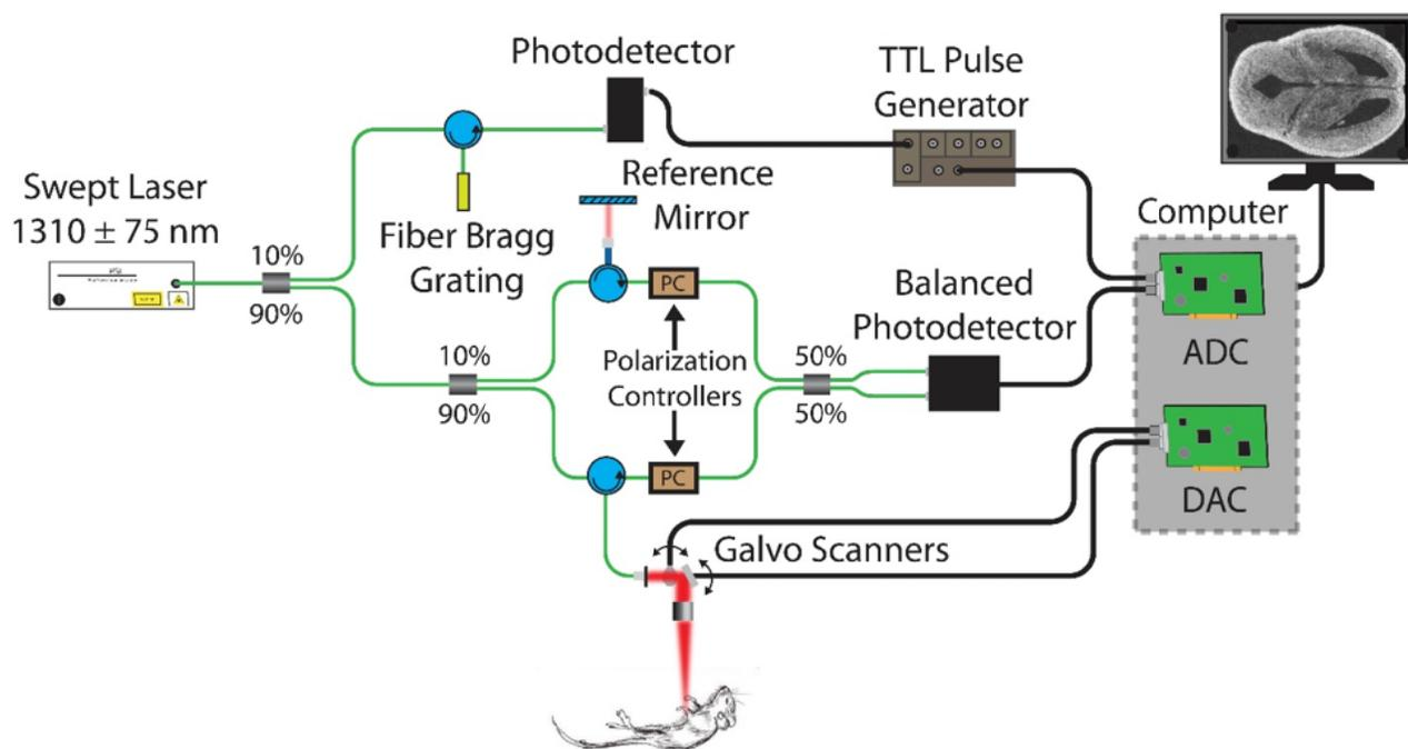
Figure 1. Schematic of the experimental setup. ADC: analog to digital converter; DAC: digital to analog converter
