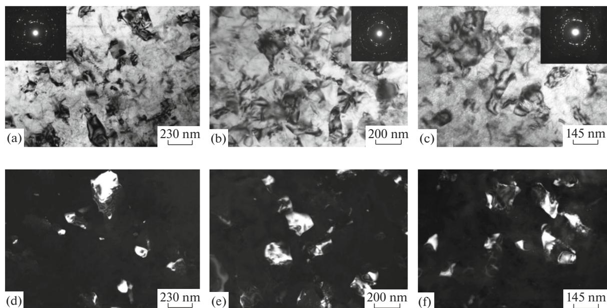
**Fig. 1.** Structure of alloy A5083 after HPT: (a, b, c) bright-field images with microdiffraction pattern; (d, e, f) dark-field images in matrix reflexes; (a, d)  $e = 7.0$ ; (b, e)  $e = 8.6$ ; (c, f)  $e = 9.3$ .
