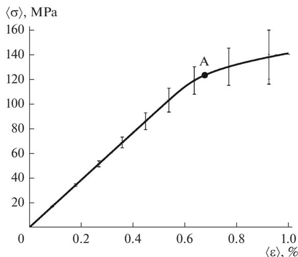
**Fig. 3.** Stress-strain diagram of zirconium ceramic–cortical bone tissue biocomposite.
