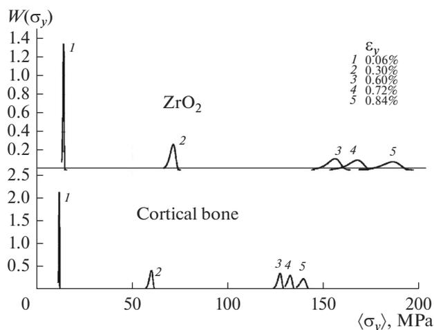
**Fig. 4.** Weibull density distribution functions of stresses  $\sigma_y$  of the ceramic and cortical bone at various effective strain values.
