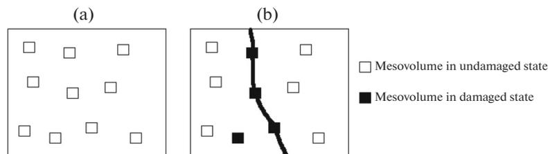
**Fig. 2.** Diagram of the employment of the percolation criterion at the macroscale: (a) set of mesovolumes in “initial state” (undamaged) and (b) formation of a joint cluster of damage.
