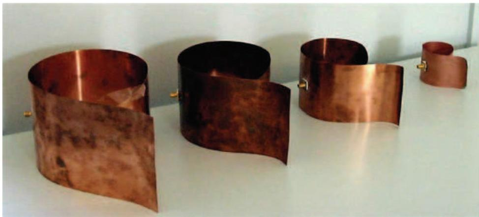
**Fig. 8.9** UWB antennas of snail type
