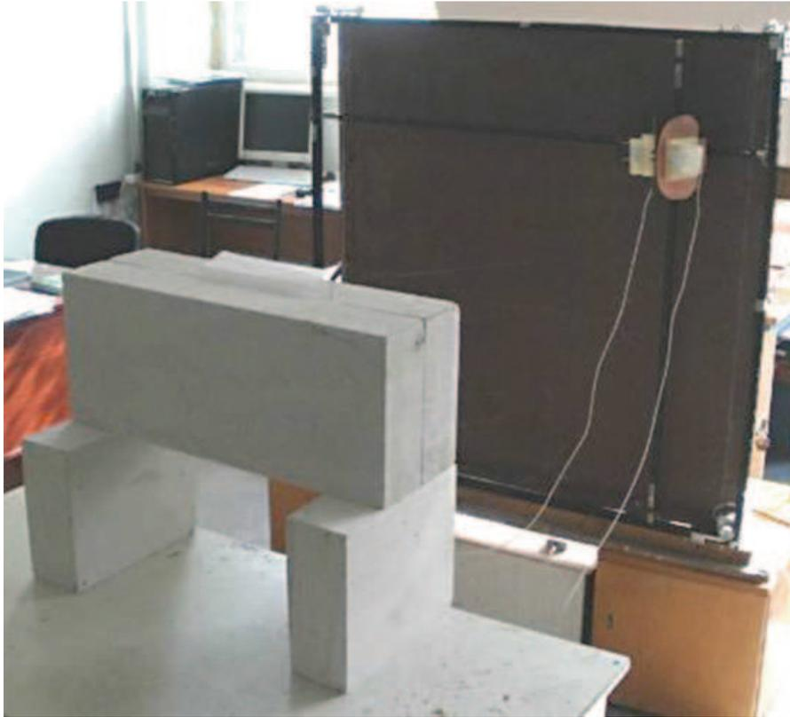
**Fig. 8.6** Scanner for UWB measurements
