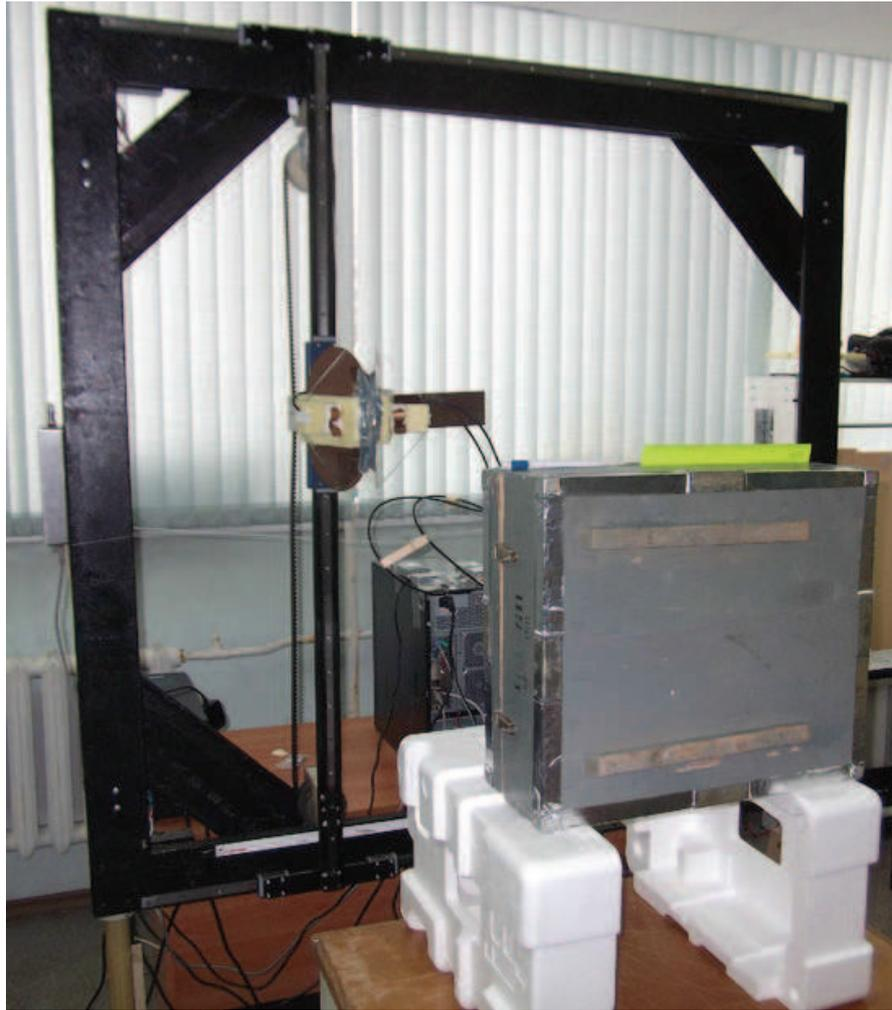
**Fig. 8.17** UWB scanner and carrying box
