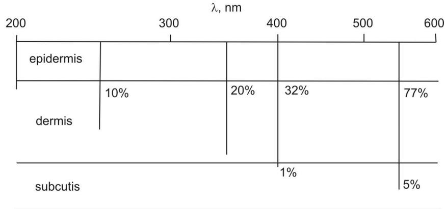
Figure 1. Light penetration depth in the skin layers as a function of radiation wavelength.
