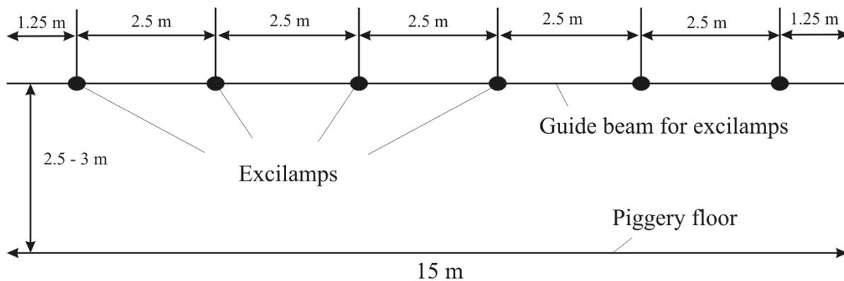
Figure 3. Arrangement of excilamps rated at irradiation of about 25–30 animals.
