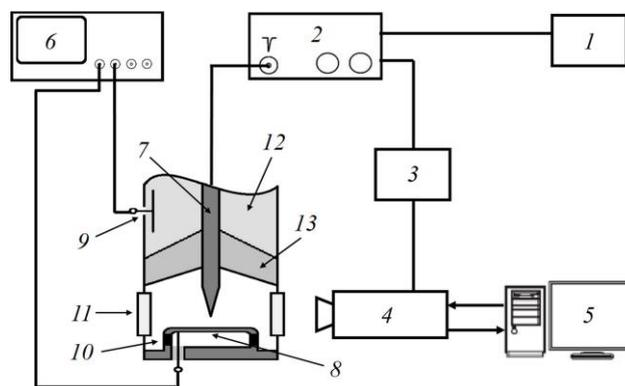
**Figure 1.** Block-scheme of the experimental setup. 1 – triggering pulser, 2 – high-voltage pulser, 3 – delay pulser, 4 – ICCD camera or streak camera, 5 – computer, 6 – oscilloscope, 7 – high-voltage electrode, 8 – grounded electrode, 9 – capacitive voltage divider, 10 – current viewing resistor, 11 – window, 12 – transmission line, 13 – insulator.
