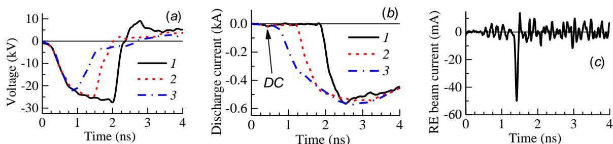
**Figure 2.** Waveforms of voltage (a), discharge current (b), as well as RE beam current pulses (c). A RE beam was registered behind the 10- $\mu$ m-Al anode. Nitrogen pressure is 100 kPa.  $d$  is 3 mm. 1, 2, 3 – different discharge implementations. Positive surges on the voltage pulses are caused by the insufficient value of  $RC$ -constant of CVD.  $DC$  – displacement current.
