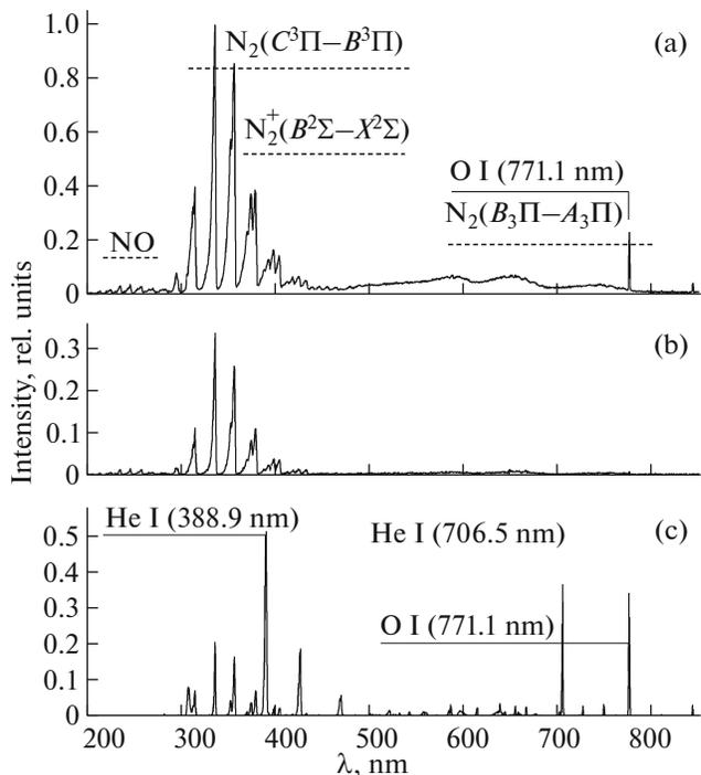
**Fig. 4.** The radiation spectra of the pulse discharge channel at  $h = 0$  mm (a), offshoot  $h \sim 20$  mm (b) and helium plasma jet (c) at  $d = 9.2$  mm,  $h = 20$  mm,  $f = 49$  kHz.
