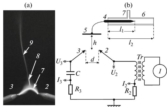
**Fig. 1.** The external form of the discharge initiating the formation of the apokamp (a) and the experimental setup (b): 1—the source of impulse voltage of positive polarity; 2—electrode; 3—electrode which is grounded through the capacitance  $C = 11.65$  pF; 4—rod electrode; 5—round current collector; 6—quartz tube with gas inlet; 7—pulse-periodic discharge channel; 8—bright offshoot; 9—apokamp; and  $R_2 = 3.6 \Omega$ ;  $R_3 = 1 \Omega$ ;  $l_1 = 75$  mm;  $l_2 = 100$  mm.
