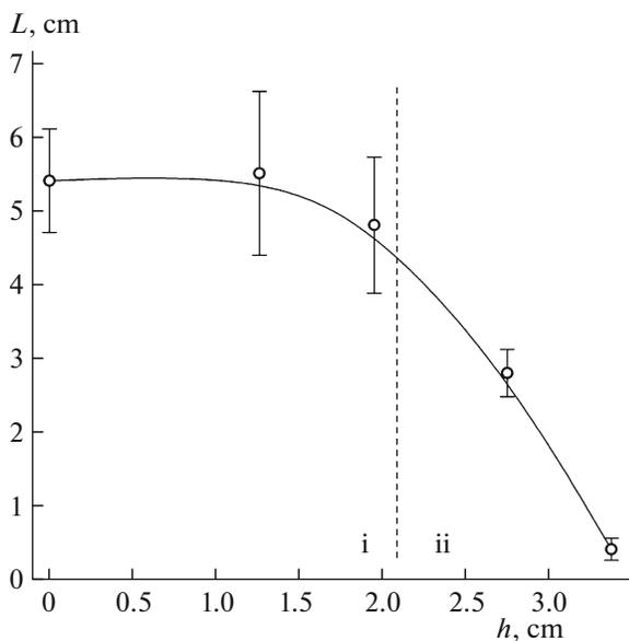
**Fig. 3.** Dependence of the length of the helium plasma jet  $L$  on the distance  $h$  at  $d = 9$  mm,  $f = 49$  kHz: (i) the zone in which the length of the helium jet varies slightly; (ii) the zone in which the length of the jet is significantly reduced.
