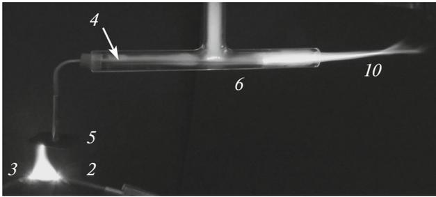
**Fig. 2.** The experimental setup during the tests: 2–4—electrodes; 5—current collector; 6—quartz tube which is filled with helium; and 10—helium plasma jet.
