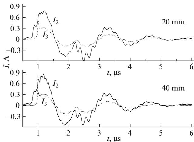
**Fig. 5.** The dependance of the current value on time at  $d = 9.2$  mm,  $h = 10$  mm, and  $f = 53$  kHz.
