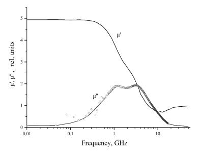
Fig.1 – The spectrum of the magnetic permeability of composite
