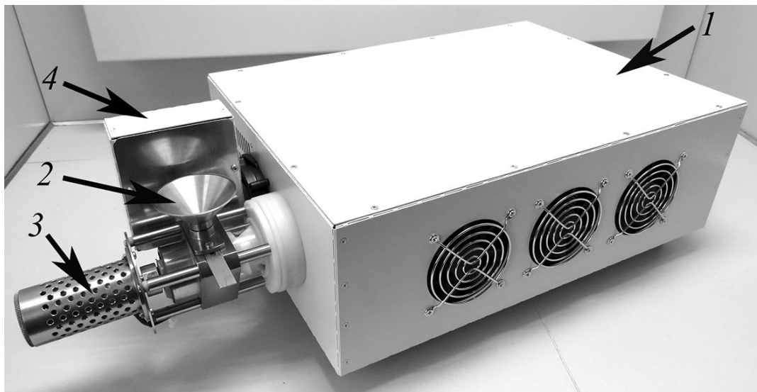
Figure 2. Setup with enhanced efficiency for internal seed irradiation: 1 – excilamp case with cooling system; 2 – seed funnel; 3 – reducer-drive for seed supply; 4 – control unit
