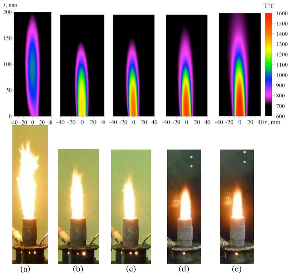
**Figure 2.** Thermograms of flame and the photographs for different steam flow rates (at a constant temperature steam  $T_v \sim 250$  °C:  $\gamma = 0.24$  (a),  $\gamma = 0.34$  (b),  $\gamma = 0.44$  (c),  $\gamma = 0.50$  (d),  $\gamma = 0.56$  (e), and a steam pressure in the range of  $8 \pm 2$  atm, respectively)
