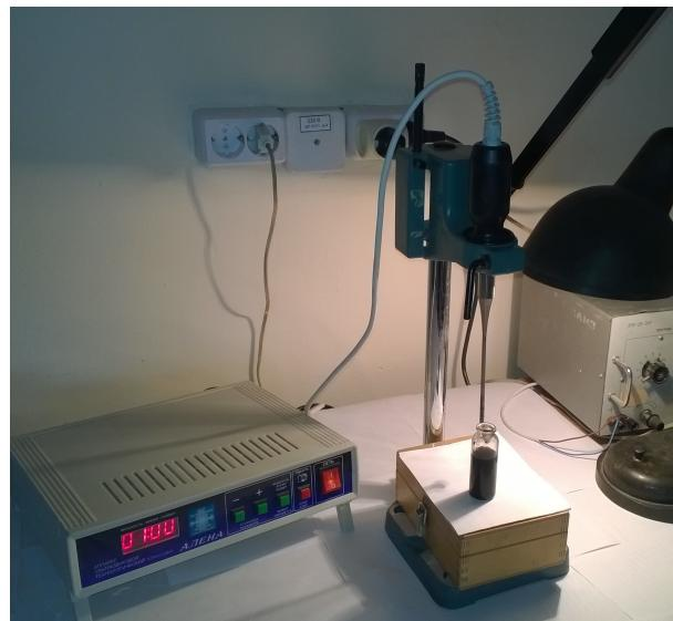
Fig. 1. Experimental ultrasonic system to dispersing MWCNT.
