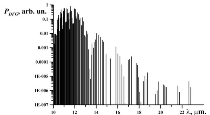
Fig. 1. Calculated spectrum of DFG at phase-matching angle 33.1°.
