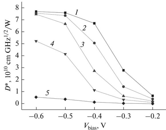
**Fig. 2.** Calculated detectability of the  $nBn$  photodetector considered in [4] as a function of the external bias at various compositions of the contact layer:  $x_{\text{cont}} = (1) 0.2$ , (2) 0.25, (3) 0.3, (4) 0.35, and (5) 0.4.
