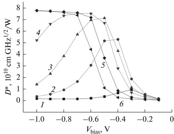
**Fig. 1.** Calculated detectability of the  $nBn$  photodetector considered in [4] as a function of the external bias at various compositions of the barrier layer:  $x_{\text{bar}} = (1) 0.45$ , (2) 0.5, (3) 0.525, (4) 0.55, (5) 0.6, and (6) 0.65.
