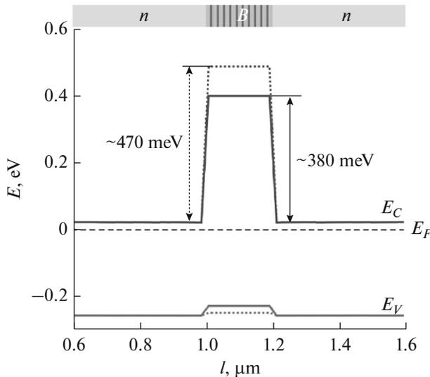
**Fig. 3.** Calculated energy band diagrams of the structures with barriers in the form of a type-III superlattice (T3SL) at a temperature of 80 K under the zero external bias [8] for two superlattice configurations. Solid and dashed curves correspond to structures 6/28 and 5/28, respectively.
