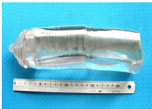
Fig. 2. ZnWO_4 crystal grown by LTG Cz technique (NIIC SIB RAS, Novosibirsk)
