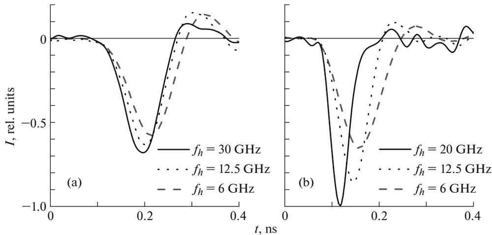
**Fig. 2.** Beam-current profiles recorded with oscilloscopes no. 1 ( $f_h = 6$  GHz), no. 2 ( $f_h = 12.5$  GHz), no. 4 ( $f_h = 20$  GHz), and no. 6 ( $f_h = 30$  GHz) for collectors (a) *A* and (b) *B*.
