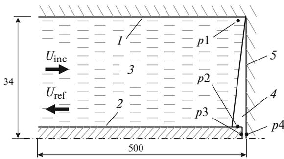
**Fig. 4.** Geometry of the calculation model of the coaxial transmission line and the gas-filled diode of the SLEP-150M generator: (1) outer electrode of the coaxial line; (2) inner electrode of the coaxial line (cathode); (3) transformer oil; (4) diode interelectrode gap; (5) anode; and (p1–p4) test points.
