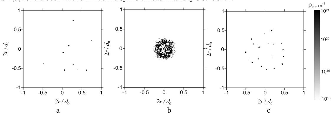
Figure 7. Cross-section profile of the volume concentration  $\rho_e$  of a plasma channel in the case of laser beam filamentation with  $E_0 = 80 \text{ mJ}$  and  $d_0 = 4 \text{ cm}$  for  $f =$  (a)  $-150$  and (b)  $+25$  m; (c) collimated beam.
