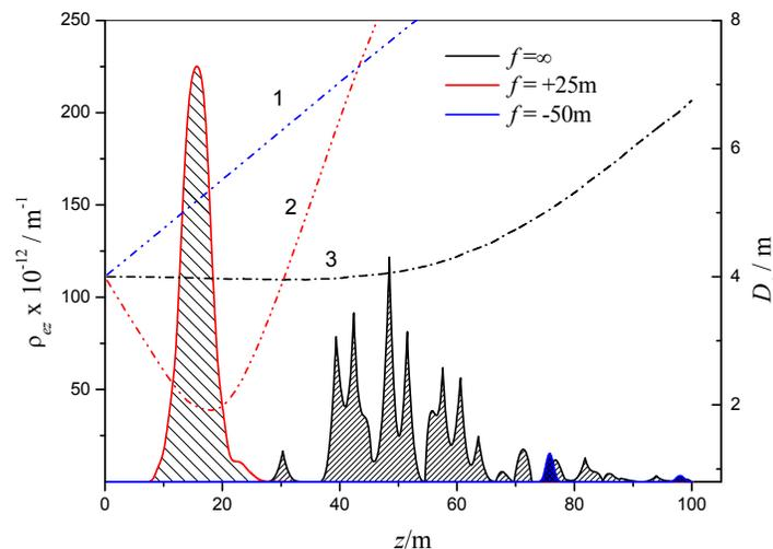
Figure 5. Path evolution of the linear concentration of free electrons (shaded areas) generated due to filamentation of the laser beam with  $E_0 = 80 \text{ mJ}$  and  $d_0 = 4 \text{ cm}$  and effective diameter  $D_e$  (curves) at  $f = (1) -50$  and  $(2) +25 \text{ m}$ ;  $(3)$  collimated beam.
