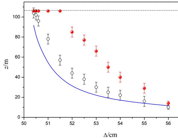
Figure 2. Coordinates of the beginning (○) and end (●) of the filamentation domain ( $E_0 = 60$  mJ,  $d_0 = 4$  cm) vs. the length of the telescope base  $D$  (focal length). Dashed curve refers to the boundary of the optical path, solid curve corresponds to the calculation by formula (1).
