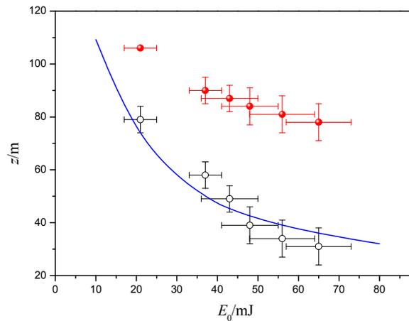
Figure 3. Coordinates of the beginning (○) and end (●) of the filamentation domain for the collimated beam with  $d_0 = 2.5$  cm vs. the laser pulse energy  $E_0$ . Solid curve corresponds to the calculation by formula (2).
