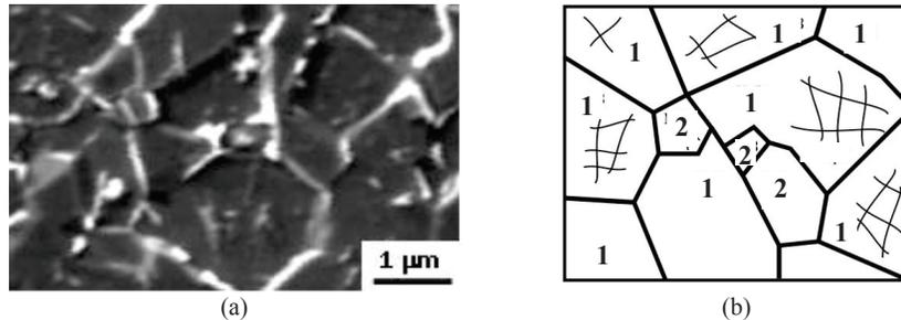
**FIGURE 1.** Grained structure after the ion implantation: a - TEM image; b - its schematic view (1 – coarse grains; 2 – small grains)
