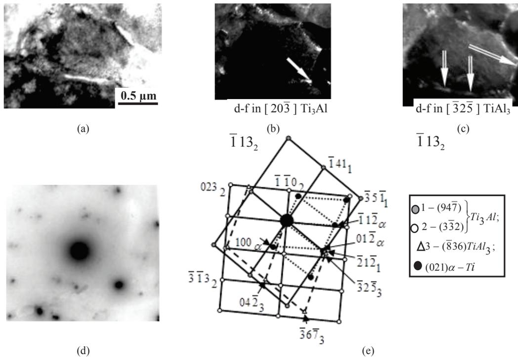
**FIGURE 3.**  $Ti_3Al$ ,  $TiAl_3$  phase precipitation in  $\alpha$  Ti grain. Electron microscope images: a – bright-field image; b, c – dark-field images obtained in  $Ti_3Al$  and  $TiAl_3$  phase reflections respectively; d, e – micro-diffraction pattern of (a) and its visual display
