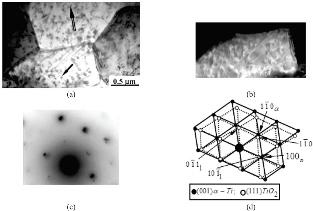
**FIGURE 4.**  $TiO_2$  phase precipitation in  $\alpha$  Ti grain. Electron microscope images: a – bright-field image (single arrow is for rounded and double arrow is for lamellar  $TiO_2$  particles); b – dark-field image obtained in  $\alpha$ -Ti and  $TiO_2$  phase reflections; c, d – micro-diffraction pattern and its visual display
