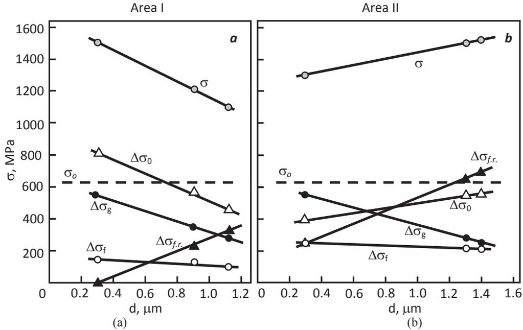
**FIGURE 6.** Dependence of the yield stress and certain hardening mechanisms contribution upon  $\alpha$ -Ti grain size across the ion-alloyed Ti layer: *a* – area I; *b* – area II;  $\sigma_0$  - yield stress of the original alloy
