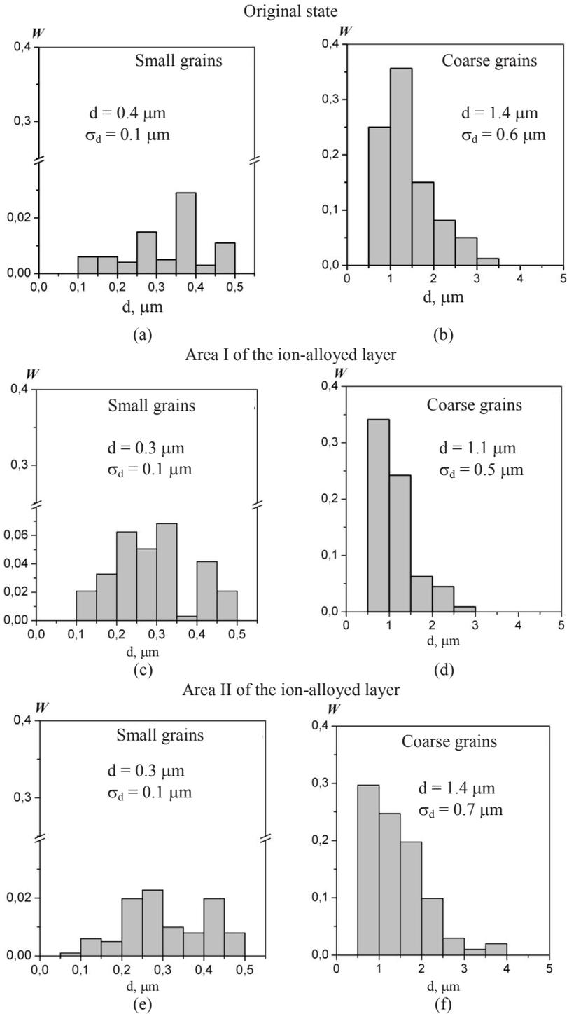
**FIGURE 2.** Grain-size distribution: a, b – original state; c, d – in ion-alloyed area I; e, f – in ion-alloyed area II
