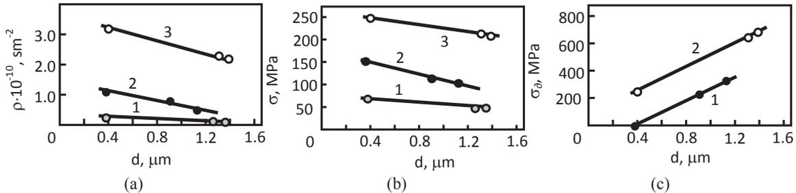
**FIGURE 5.** Dependences of scalar density (a), shear stresses (b), and local stresses (c) and the average grain size  $\alpha$ -Ti before and after ion implantation: 1 – original Ti specimen; 2 – ion-alloyed layer in area I; 3 – surface layer of the area II
