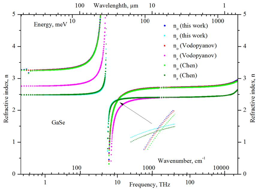
Figure 2. Comparison calculated refraction indices for GaSe crystal.
