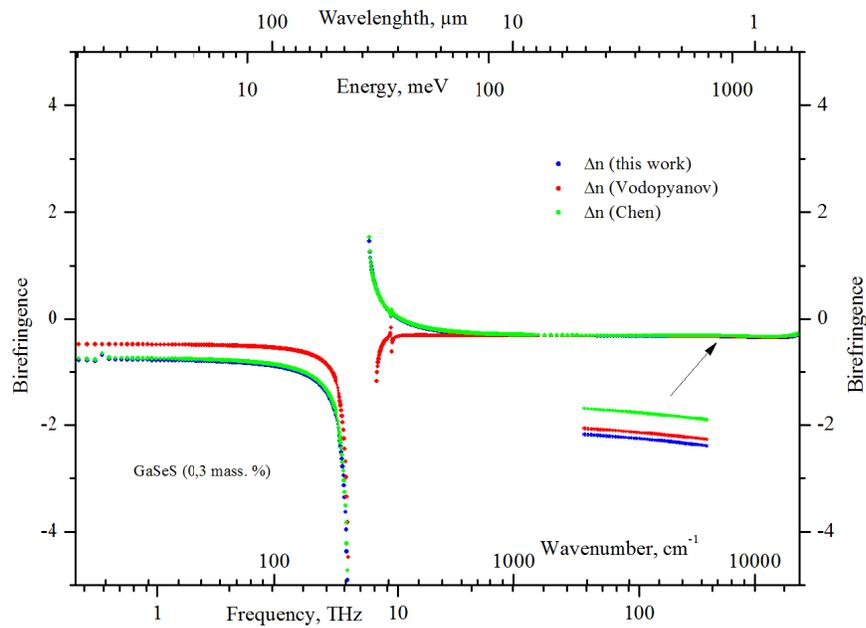
Figure 5. Comparison calculated birefringence for GaSeS (0.3 mass.%) crystal
