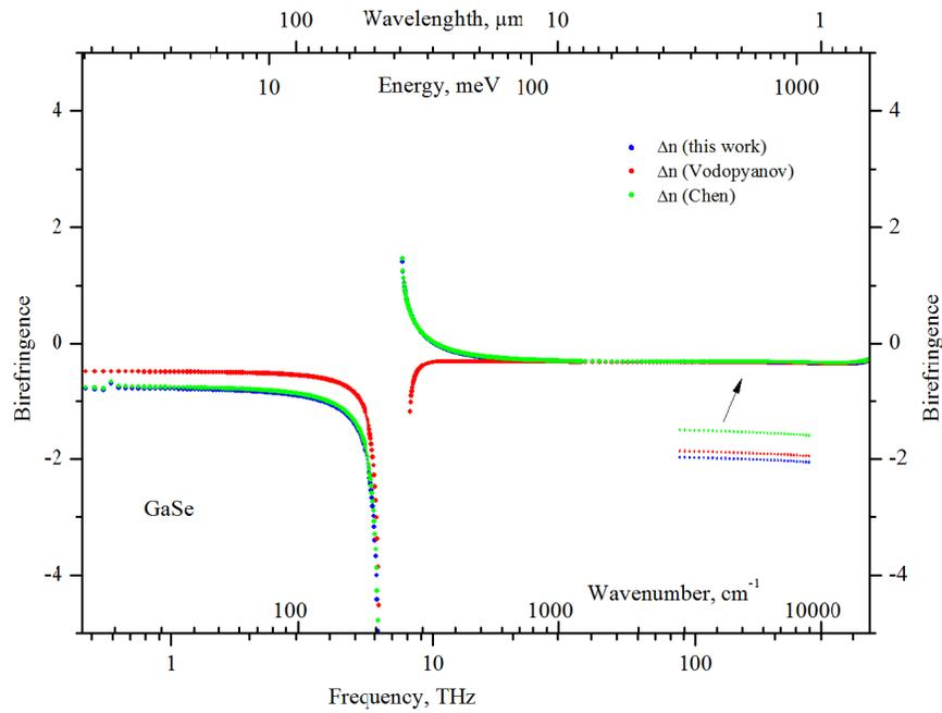
Figure 4. Comparison calculated birefringence for GaSe crystal
