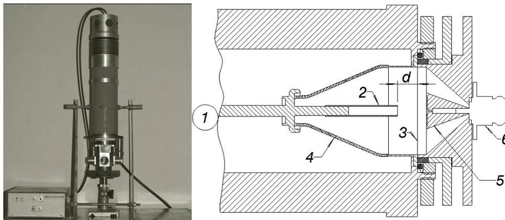
Figure 1. (a) - A setup with the discharge chamber and generator RADAN-220. (b) - Schematic diagram of the gas-filled diode and collector assembly: (1) connection to a high-voltage pulse generator; (2) cathode; (3) foil anode; (4) insulator; (5) cone-shaped collector; (6) connecting socket.
