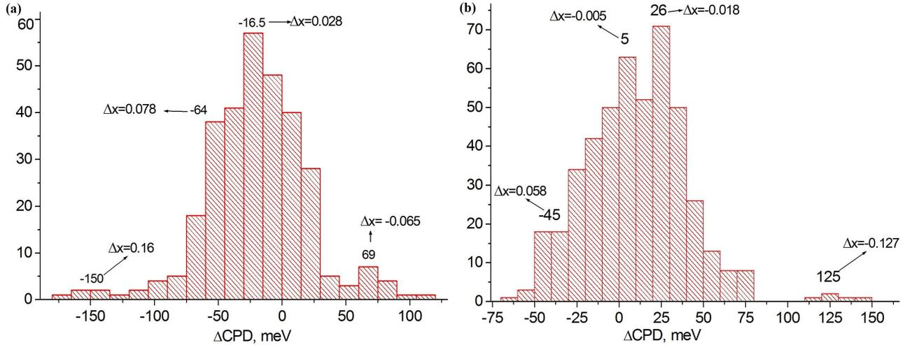
Figure 4 Distribution of the deviation of the CPD value of individual crystal grains of a V-defect versus the CPD of the epitaxial film: a) original film; b) after irradiation, 1 – distribution of  $\Delta CPD$ , 2 – assemblage of normal distributions, 3 – combined distribution; the arrows indicate the variation  $\Delta x$  of the CdTe content for the given value of  $\Delta CPD$ .
