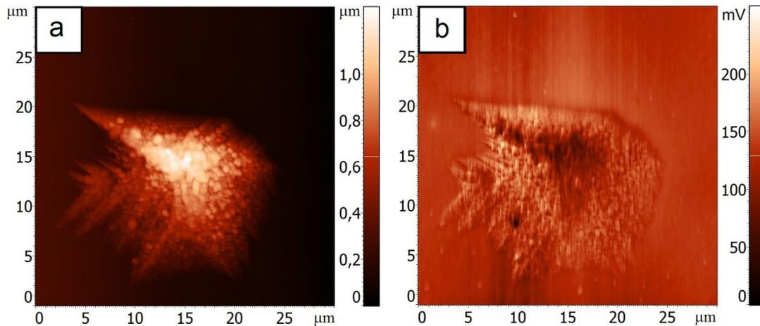
Figure 3 AFM image of a V-defect surface morphology (a) and the distribution of the surface potential or CPD (b).
