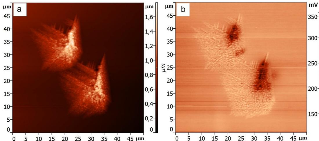
Figure 2 AFM image of morphology (a) and CPD (b) of the MCT epitaxial film in the vicinity of a V-defect.
