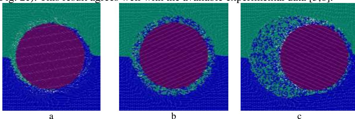
Figure 2. Structure of the material in the vicinity of the rotating tool at different points of time,  $V_{trans} = 0.2$  m/s and  $V_{rot} = 7.6$  m/s:  $t=0.0004$  s (a),  $t=0.015$  s (b),  $t=0.07$  s (c).
