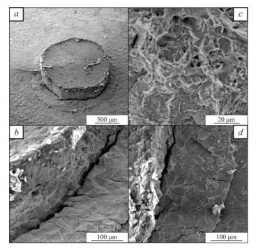
FIGURE 2. Failure of the welded joint of titanium alloy VT6 in the nanostructured initial state (a), characteristic structure of the main zones of the sample fracture (b), ductile (pit) fracture in the zone A (c), intercrystallite fracture in the zone B (d)
