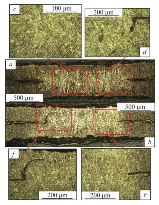
FIGURE 1. Cross-section of studied samples (a, b), the metal structure in the central region (c), pores in the contact zone (d), discontinuities along edges of the contact (f, e)
