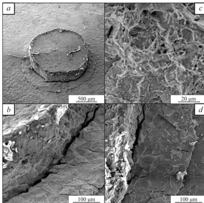
**FIGURE 2.** Failure of the welded joint of titanium alloy VT6 in the nanostructured initial state (a), characteristic structure of the main zones of the sample fracture (b), ductile (pit) fracture in the zone *A* (c), intercrystallite fracture in the zone *B* (d)
