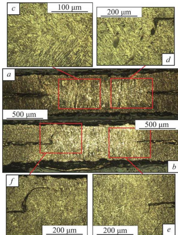
**FIGURE 1.** Cross-section of studied samples (a, b), the metal structure in the central region (c), pores in the contact zone (d), discontinuities along edges of the contact (f, e)
