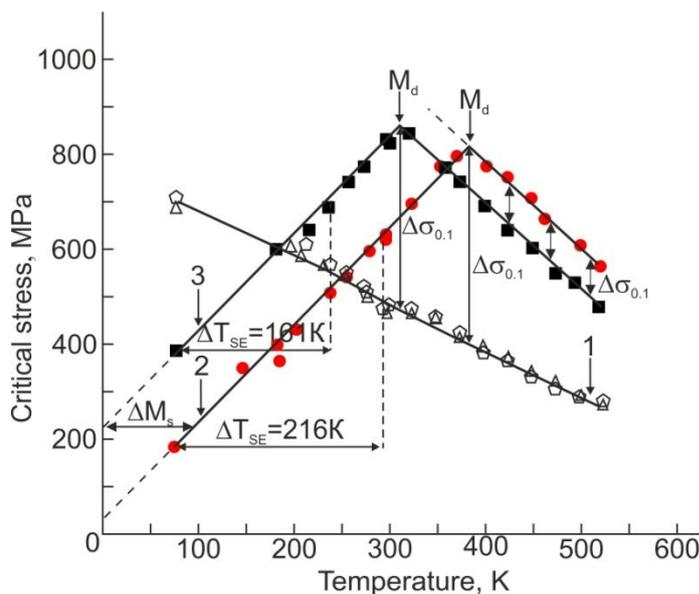
**Figure 1.** Temperature dependence of critical stresses  $\sigma_{cr}$  for [001] single crystals FeNiCoAlNb(B) alloys at tensile deformation: curve 1 – single-phase state after quenching; the curve 2 – the FeNiCoAlNb crystals, aged at  $T = 973$  K, 5 hours; curve 3 – FeNiCoAlNbB crystals, aged at  $T = 973$  K, 5 hours.
