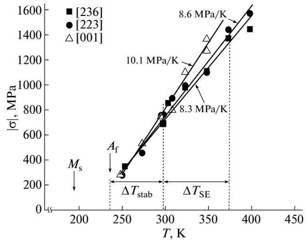
**Fig. 2.** Temperature dependences of the critical stresses of martensite formation in compression-strained  $\text{Ni}_{51.0}\text{Ti}_{36.5}\text{Hf}_{12.5}$  single crystals oriented along [001], [236], and [223] directions: ( $\Delta T_{\text{stab}}$ ) temperature interval of stress-induced martensite stabilization; ( $\Delta T_{\text{SE}}$ ) temperature interval of SE.
