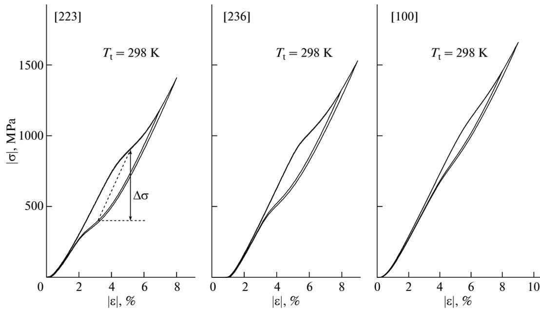
**Fig. 3.** Stress–strain curves  $\sigma(\varepsilon)$  measured at  $T_t = 298$  K in compression-strained  $\text{Ni}_{51.0}\text{Ti}_{36.5}\text{Hf}_{12.5}$  single crystals oriented along [223], [236], and [001] directions.
