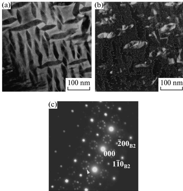
**Fig. 1.** Microstructure of as-grown  $\text{Ni}_{51.0}\text{Ti}_{36.5}\text{Hf}_{12.5}$  single crystals: (a, b) bright-field and dark-field TEM images, respectively; (c) the corresponding selected area diffraction pattern, zone axis is  $[001]_{\text{B}2}$ ; the dark-field image was recorded using the reflection indicated by the arrow in the diffraction pattern.
