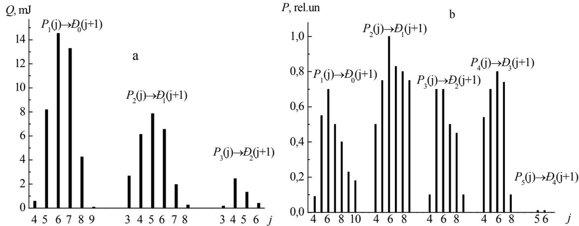
Figure 6. Energy (a) and intensity (b) lasing line distributions of a non-chain (a) HF and (b) DF laser pumped by REP DD, SF<sub>6</sub> : H<sub>2</sub>(D<sub>2</sub>) = 240 : 30 Torr mixture is used. CaF<sub>2</sub> (a) and Ge (b) plates are used as exit mirrors of the laser cavity.
