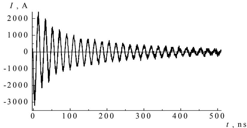
Figure 2. Waveform of the short-circuit current in the laser gap.
