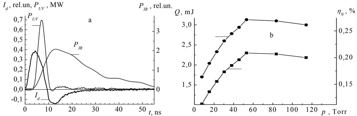
Figure 4. Oscillograms of REP DD current pulses and generation in the mixture  $N_2:SF_6=300:45$  Torr on the first ( $P_{IR}$ ) and second ( $P_{UV}$ ) positive bands of nitrogen (a) and dependences of radiation energy  $Q$  at  $\lambda=337.1$  nm and electrical efficiency of nitrogen laser  $\eta_0$  on pressure of  $SF_6$  at the nitrogen pressure 300 Torr (b).
