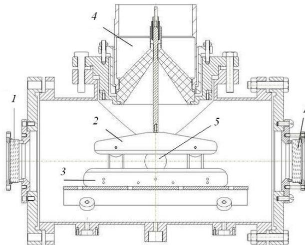
Figure 1. Schematic diagram of the laser pumped by REP DD. (1) mirrors of the laser resonator, (2, 3) blade electrodes, (4) the RADAN-220 pulse generator, (5) side window.
