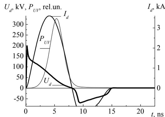
Figure 3. Calculated waveforms of the REP DD current, voltage across the laser gap and laser pulse at  $\lambda = 337, 1 \text{ nm}$  in the  $\text{N}_2 : \text{SF}_6 = 300 : 45 \text{ Torr}$  mixture.
