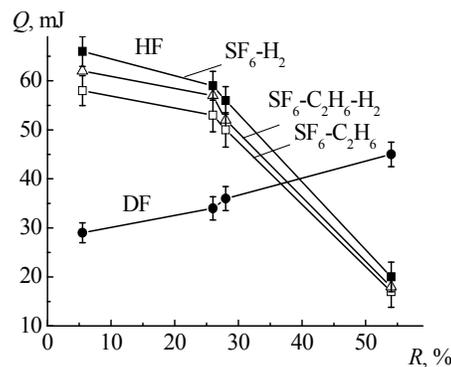
Figure 5. Output energy of laser on molecules HF and DF vs the reflection coefficient of the output mirror of cavity for the mixtures:  $SF_6:H_2(D_2)=8:1$ ,  $SF_6:H_2:C_2H_6=44:3:1$ , and  $SF_6:C_2H_6=20:1$  at the pressure of 275Torr
