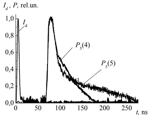
Figure 7. Oscillograms of discharge current pulses and lasing at  $P_5(4)$  and  $P_5(5)$  lines of a REP DD pumped DF laser in  $SF_6$ :  $D_2 = 240 : 30$  Torr mixture, a Ge plate is used as an exit mirror of the resonator.
