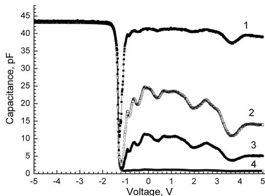
Fig. 2. CVC of MIS structure based on HgCdTe containing QW measured at 30 K at different frequencies: 1 – 1 kHz, 2 – 5 kHz, 3 – 10 kHz, 4 – 50 kHz.
