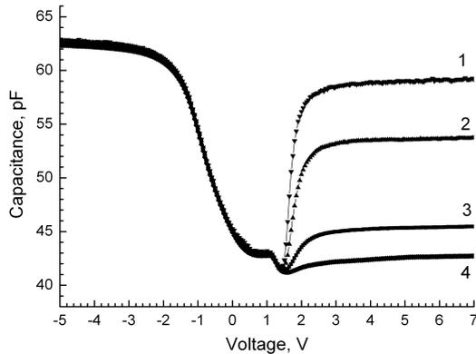
Fig. 1. CVC of MIS structure based on varyband HgCdTe without QW measured at 20 K at different frequencies: 1 – 10 Hz, 2 – 20 kHz, 3 – 50 kHz, 4 – 100 kHz.
