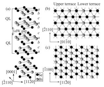
Fig. 1. (a) – Crystal structure of  $Bi_2Se_3$ , abc is the atomic layer stacking sequence. (b), (c) – Top views of the  $Bi_2Se_3$ surface containing  $[01\overline{1}0]$ -oriented (b) and  $[11\overline{2}0]$ -oriented (c) steps. The steps are marked by dashed lines
