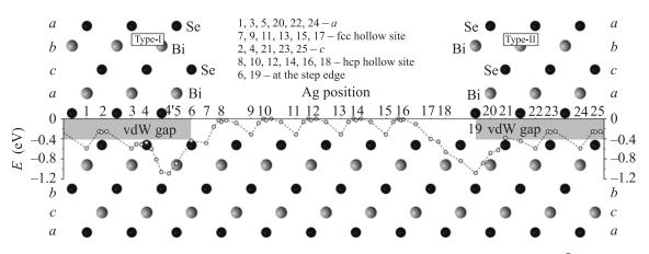
Fig. 2. The total energy as a function of the silver atom position on the surface, in the vicinity of the  $[01\overline{1}0]$ -oriented step and inside the vdW gap. Two different terminations of  $[01\overline{1}0]$ -oriented step are shown: type-I (left) and type-II (right)
