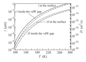
Fig. 4. The temperature dependencies of the diffusion length, l (left axis), and the diffusion coefficient, D (right axis), of the silver atom on the Bi<sub>2</sub>Se<sub>3</sub> surface and within the vdW gap estimated within 1s time window. Both dependencies drawn in logarithmic scale. The temperature range is chosen in accordance with those in available experimental works [22, 23]
