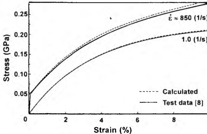
Fig. 8 Comparison of TPM results with test data
