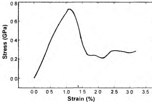
Fig. 10 Stress-strain curve from MPM calculation
