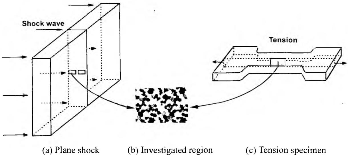
Fig. 2 Schematic of dynamically loaded specimen
