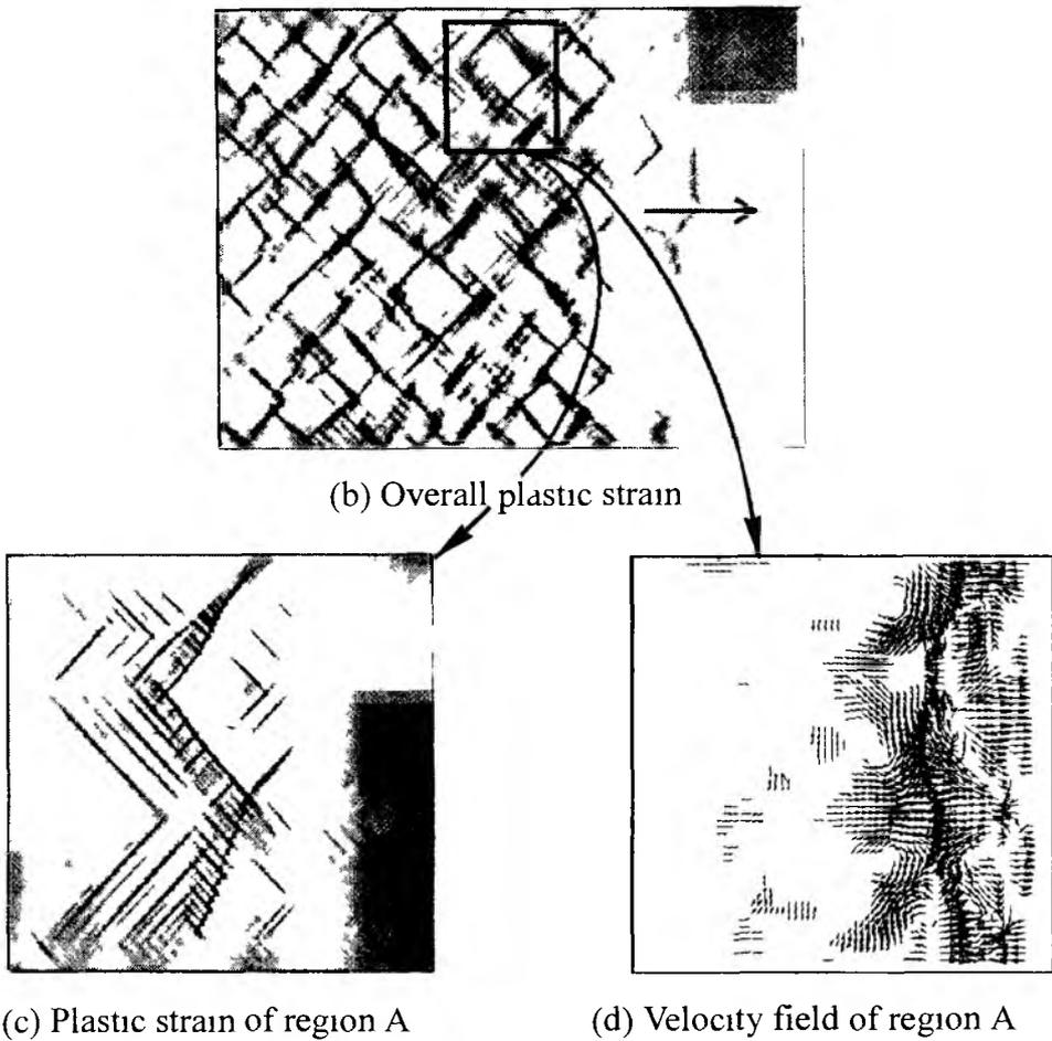
Fig 6 Plastic behavior of polycrystalline specimen under 9GPa shock from MPM calculation
