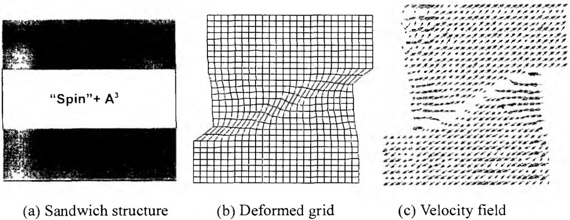
Fig. 4 Shear of sandwich structure and simulation results
