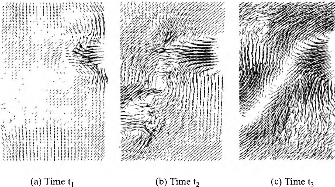
Fig. 1 Calculated velocity field of material in elastic-plastic state under tension [8]
