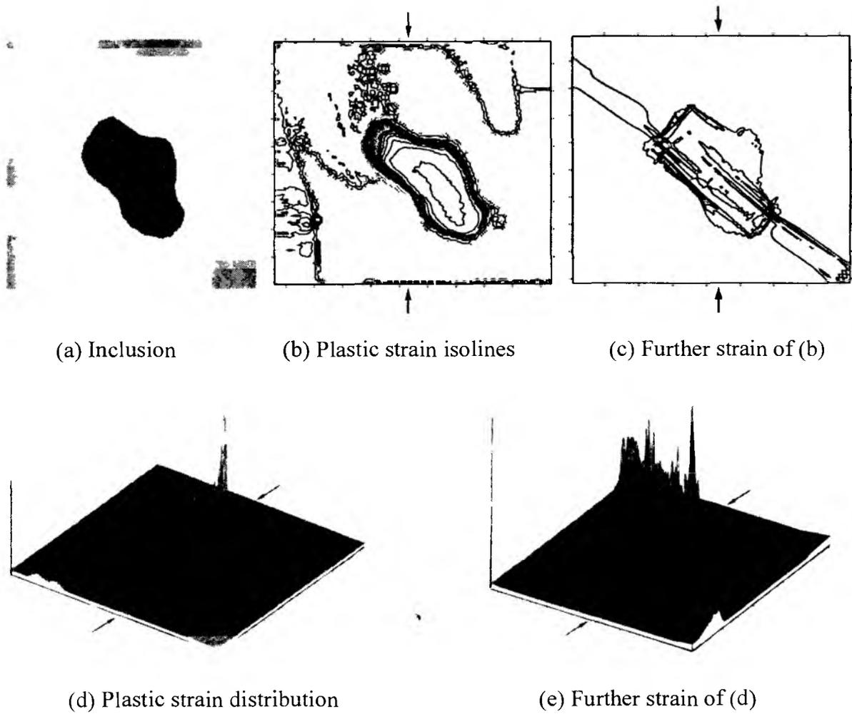
Fig. 5 Specimen under compression calculated by present model to exhibit rotation effect
