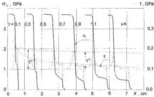
Fig. 3. The calculation of plane shock wave propagation in Al 6061-T6 with amplitude 3.7 GPa.
