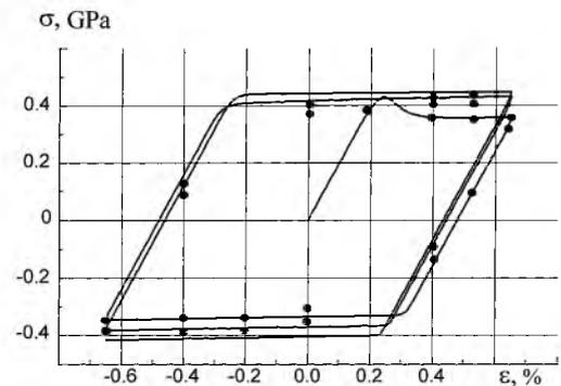
Fig. 1. Cyclic loading of the steel; • – experiment [7].
