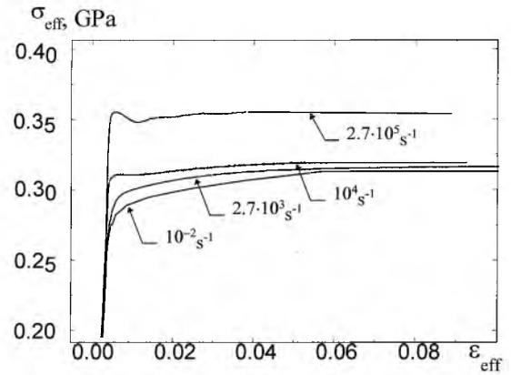
Fig. 5. Stress–strain curves of Al 6061-T6 under tension of different strain rates.
