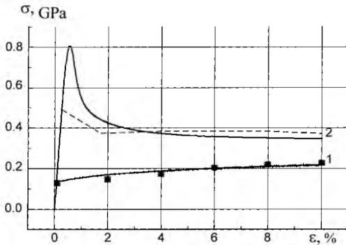
Fig. 2. Stress–strain curves for iron under different strain rates. (1)  $\dot{\epsilon} = 10^{-2} \text{ s}^{-1}$ ; (2) dynamic loading  $\dot{\epsilon} = 10^4 \text{ s}^{-1}$ . Dots and dashed lines – experiments [8].
