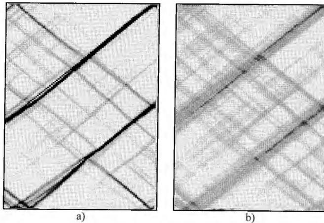
Fig. 6. Plastic strain distribution after stretching up to 3% (■ – 20%, □ – 0–0.7%) with (a)  $\dot{\epsilon} = 10^{-2} \text{ s}^{-1}$  and (b)  $\dot{\epsilon} = 10^4 \text{ s}^{-1}$ .
