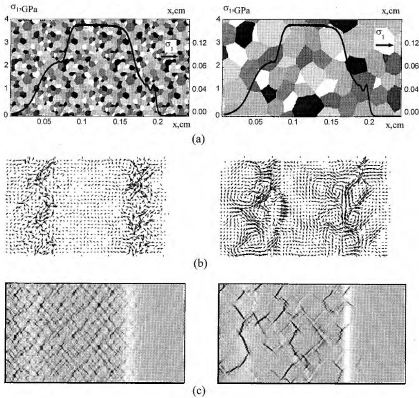
Fig. 4. Aluminium meso volumes shocked by 3.7 GPa: (a) calculated maps with different grain size (about 80 and 500  $\mu\text{m}$ ); (b) fields of particle velocities; (c) plastic strain distributions (■ – 4.5%, □ – 0–2%).
