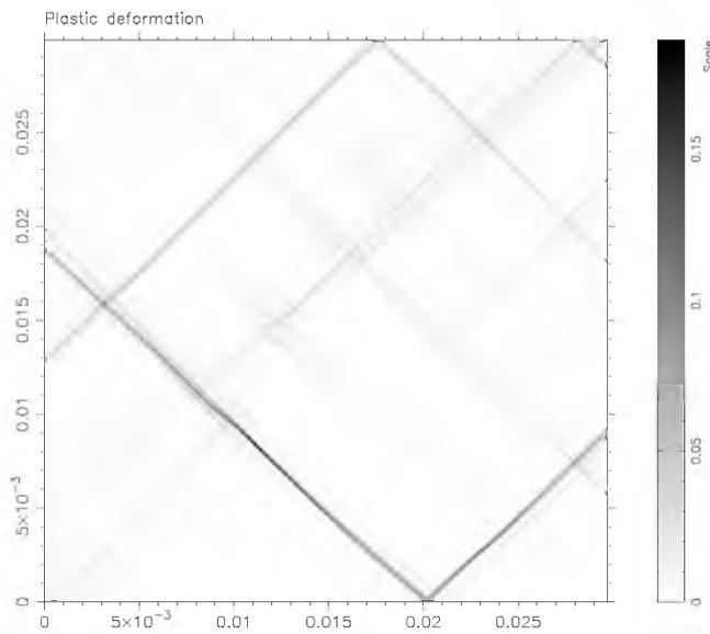
*Figure 4.* Localized strain bands in representative mesovolume.
