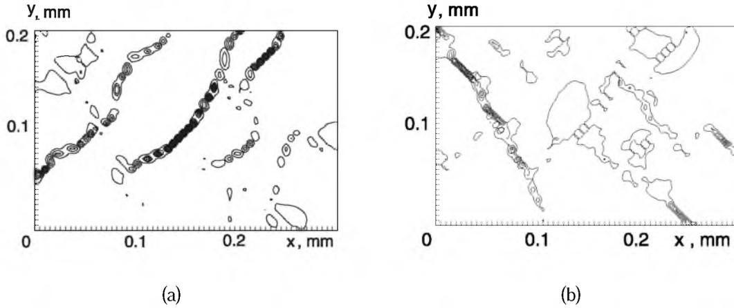
Figure 7. Contour maps for positive (a) and negative (b) values of rotations in deformed mesovolume of Al-Li alloy.
