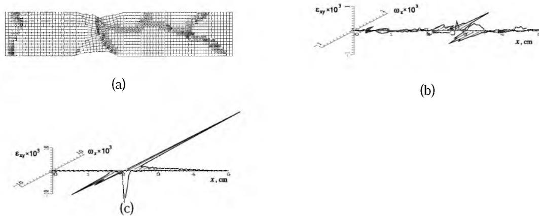
Figure 1. Calculation grid for coarse-grained Al sample with 3 percent tensile strain (a) and distribution of plastic shear and rotation along the sample axis in different time moments (b)–(c).
