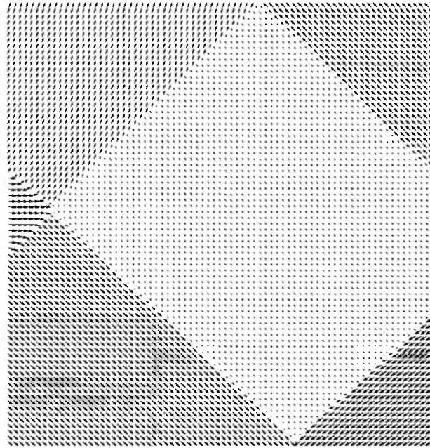
Figure 5. Velocity field in representative mesovolume at fragmentation.
