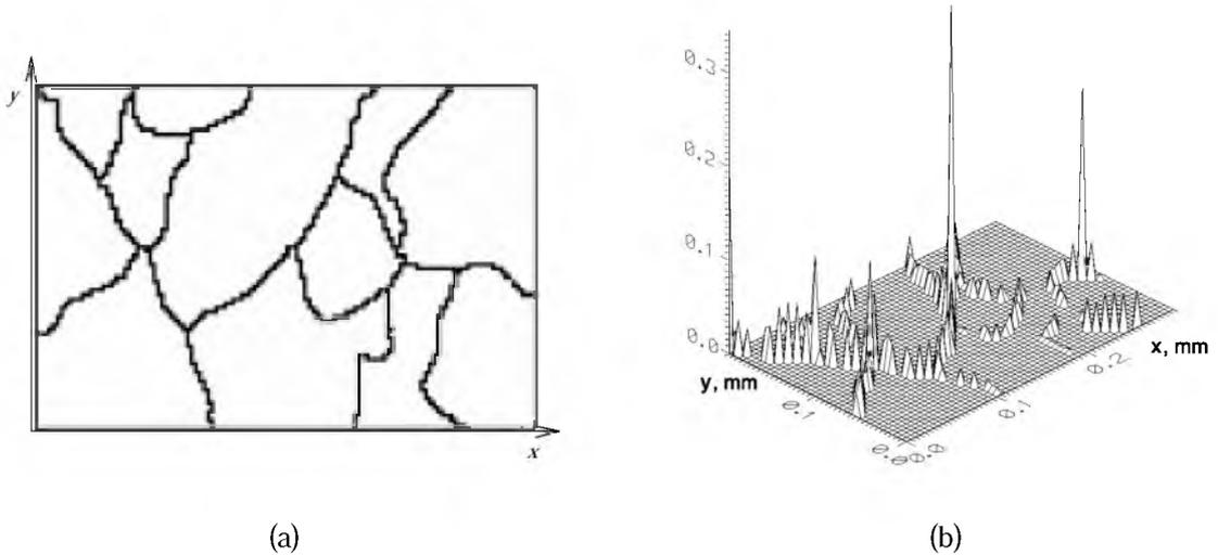
Figure 6. Reference structure of a mesovolume of Al-Li alloy (a) and space distribution of plastic energy when integral strain of the sample is 0.25 percent (b).
