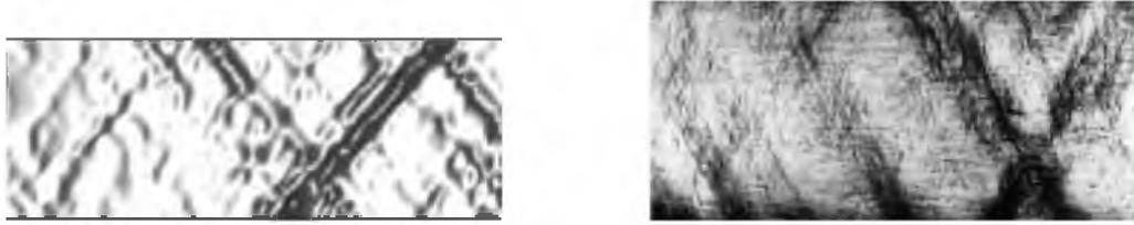
Figure 2. Mesobands of localized strain on the surface of thin steel plates. The width of the plates in both figures are equal to 1 cm.
