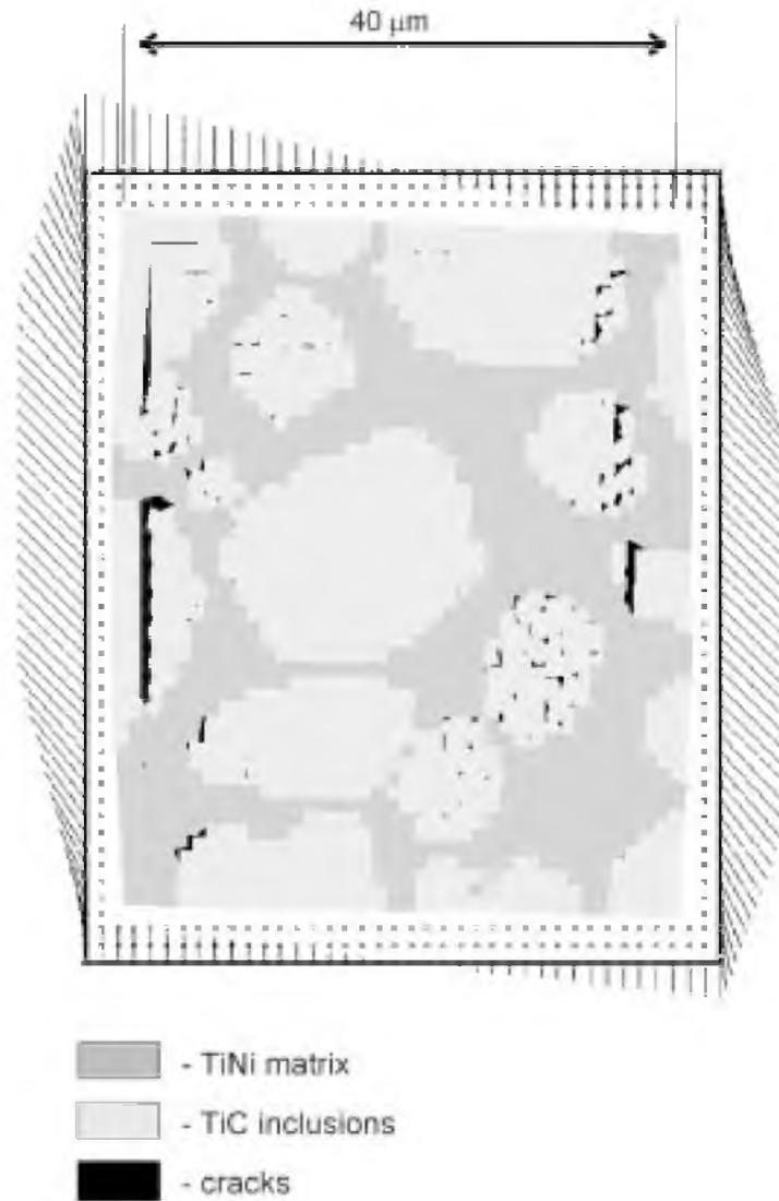
Figure 8. An example of simulation of mesocracks formation at the stage of large plastic deformation in the composite material with plastic matrix and brittle inclusions.
