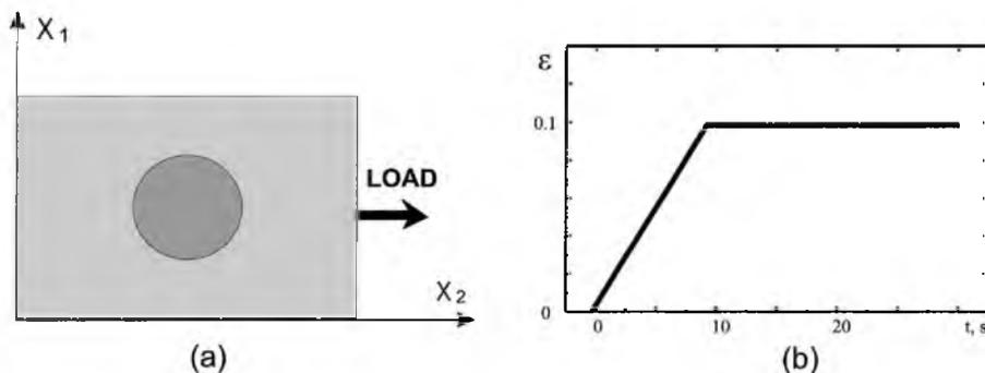
Fig. 1. The structure of viscous-elastic model sample (a) and time-dependent stretching (b).
