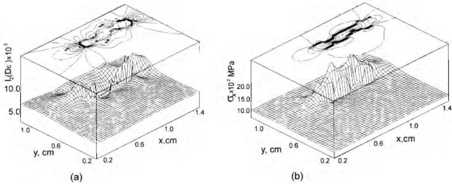
Fig. 8. Distribution of effective strains (a) and stresses (b) in the ceramic sample before cracking.
