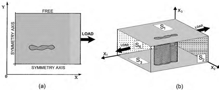
Fig. 4. Structure of the composite sample and load condition for 2D- (a) and 3D- (b) calculation.
