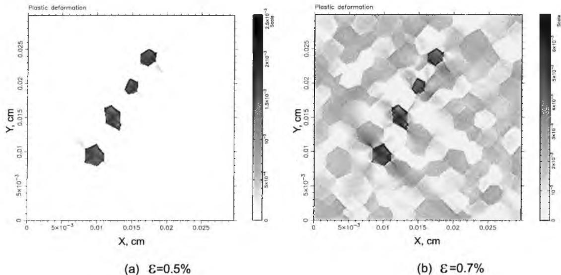
Fig. 11. Distribution of effective plastic strains in the mesovolume of polycrystalline steel.
