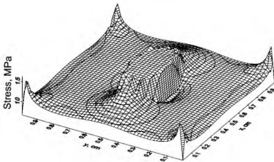
Fig. 2. Distribution of shear stresses in the heterogeneous viscous-elastic sample.
