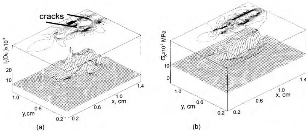
Fig. 9. Distribution of effective strains (a) and stresses (b) in the ceramic sample after cracking.
