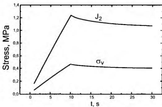
Fig. 3. Shear and cubic stress relaxation in the heterogeneous viscous-elastic sample.
