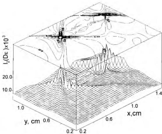
Fig. 5. Effective strains in ceramic sample with elastic perfectly-plastic matrix.
