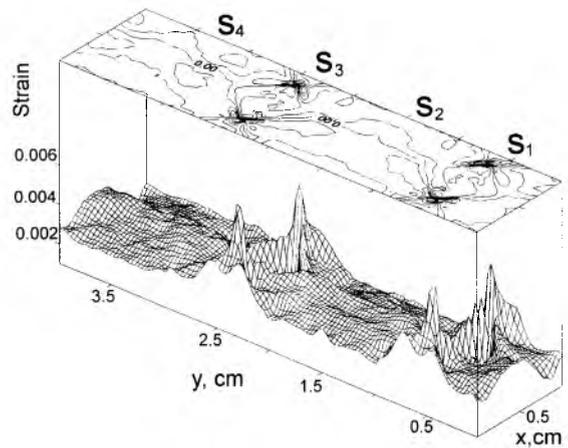
Fig. 6. Strain localisation in the ceramic sample under stretching at  $\epsilon_{11} = 0.2\%$  (3D simulation).
