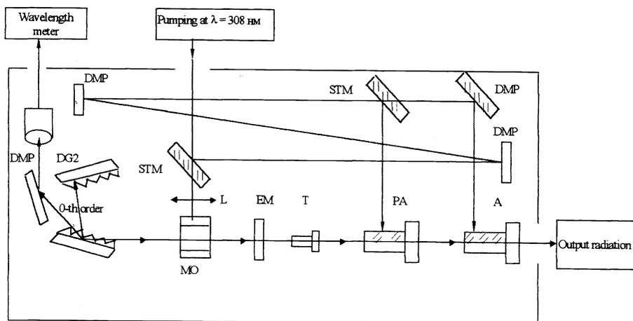
Fig. 7. Block diagram of the MZhL dye laser system. MO, PA, A are the master oscillator, preamplifier, amplifier, respectively, STM are semitransparent mirrors, DMP are total reflectors, DG1-2 are diffraction gratings, EM is the MO output mirror. T is a telescope. L is a cylindrical lens.
