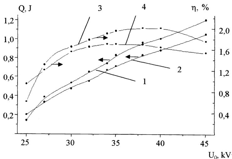
Fig. 6. Output energy (1, 2) and efficiency (3, 4) of the LIDA-3M laser as a function of charging voltage of storage capacitors.  $C_1 = 0,8 C_0$ . Gas mixture of the Xe:HCl = 18:3 Torr composition at  $p=3$  atm (2, 4) and  $p=3,5$  atm (1, 3) is used.
