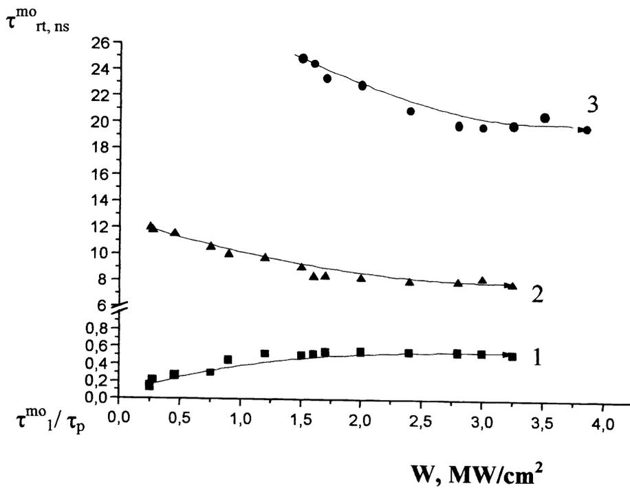
Fig.9. Ratio of the MO pulse duration to that of pumping pulse  $\tau_1^{mo}/\tau_p$  (1) and rise-time of the master oscillator pulse  $\tau_{rt}^{mo}$  (2,3) versus specific input power on the MO obtained at  $\tau_p=40$  ns (1,2) and  $\tau_p=75$  ns (3).
