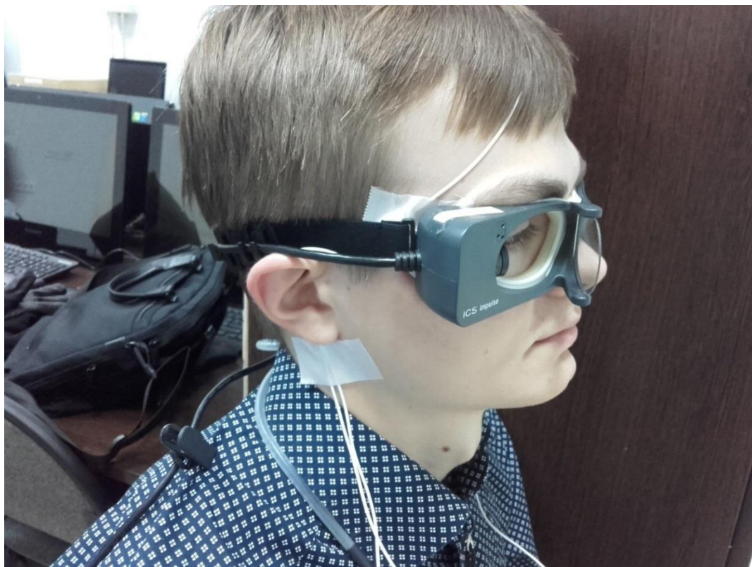
Figure 4 – Video eye tracking system placed on subject's head
